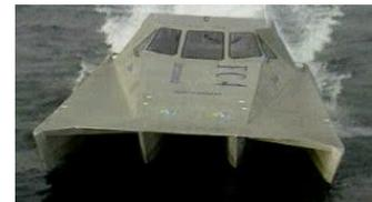
The Quadrimaran has four identical wedge-shaped planing hulls that are flat on the bottom and sloped downward toward the stern. It was designed to operate at 45-60 knots but with relatively lower drag than other high-speed ships, yielding power and fuel savings to compensate for the increases in structure and outfit from having four hulls.
