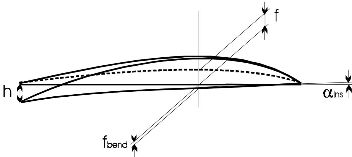
**Fig. 4 Influence of bending on the attack angle**
