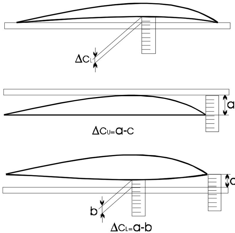
**Fig. 2 Distortions of hydrofoil profiles**
