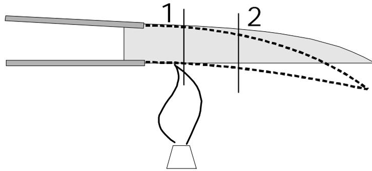
**Fig. 5 Thermal bending of a trailing edge**
