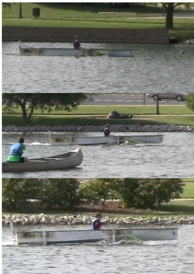
Figure 37. Hydrofoil boat in take-off and flight.
