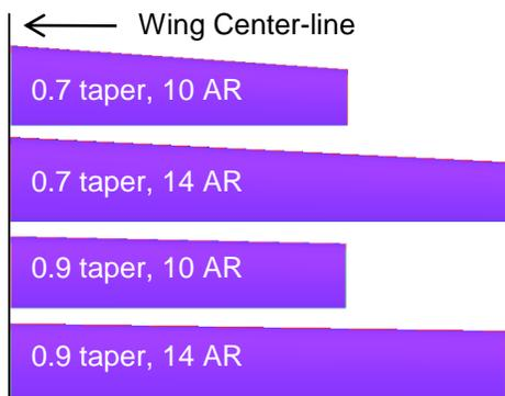
Figure 26. Representative sketches of half-wing planforms used for the single 3D foil taper and aspect ratio study.
