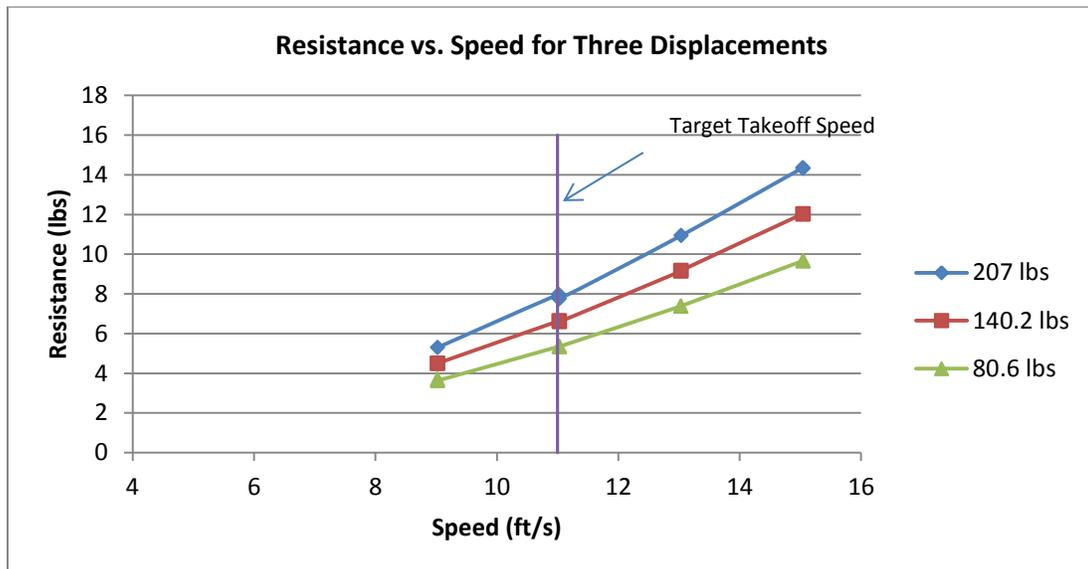
Figure 13: Results of the hull resistance tests, showing resistance vs. speed for three displacements.
