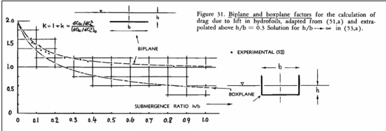
Figure 6: Hoerner's Drag plot for depth
