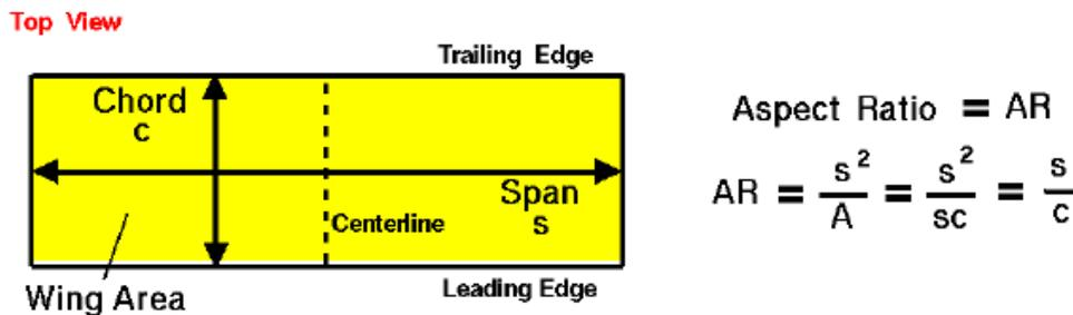
Figure 4: Diagram showing main foil dimensions
