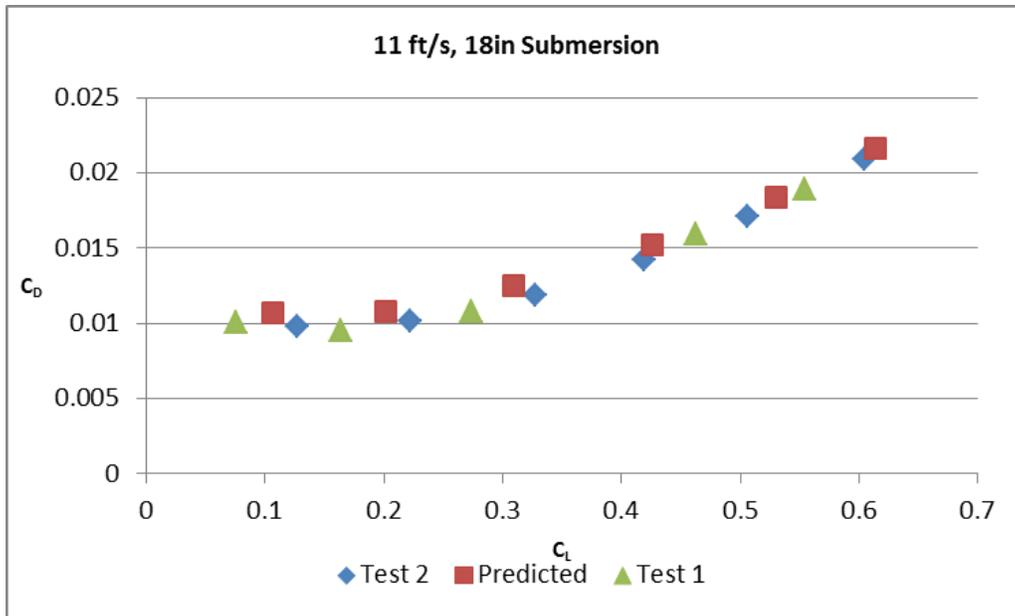
Figure 17: Comparison of foil performance to spreadsheet predictions
