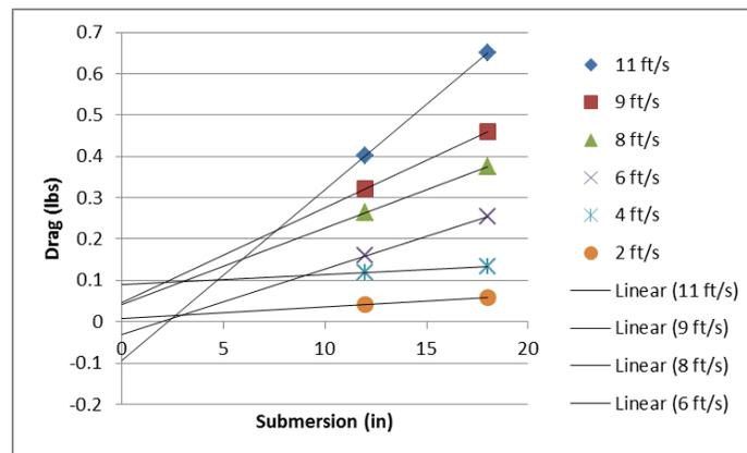
Figure 16: Drag vs. Submersion of the strut for a range of velocities.
