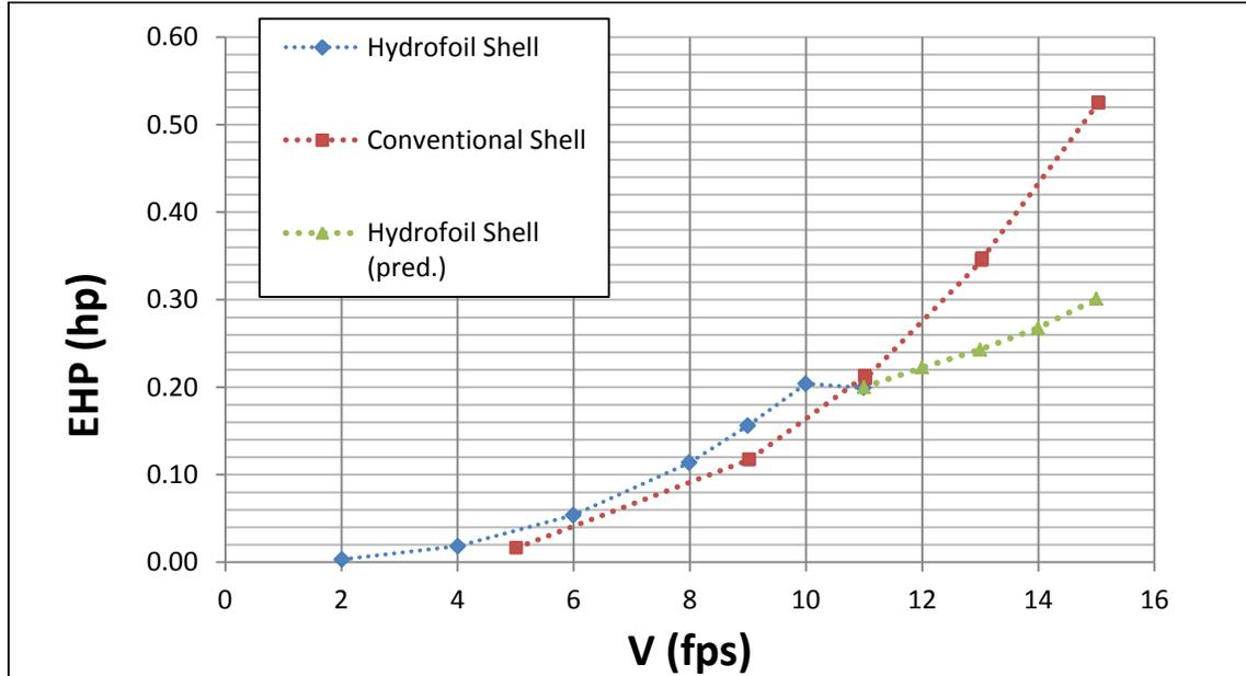
Figure 19: EHP vs. Speed for the conventional shell and the shell with hydrofoils.
