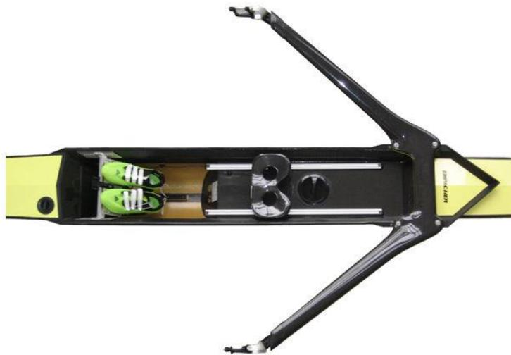
Figure 3: Picture of a traditional rigger system for a single scull.
