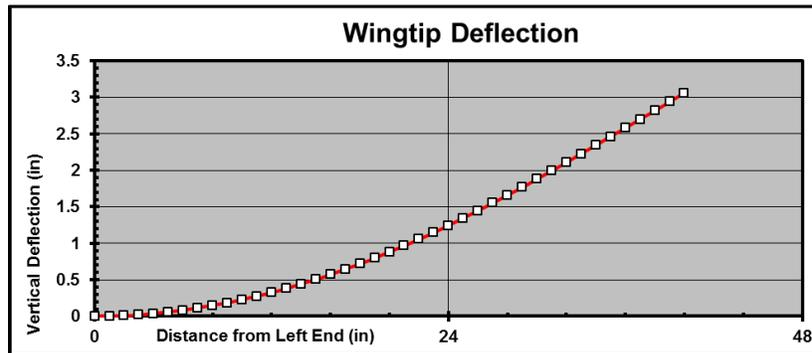
Figure 8: Plot showing modeled deflection across one half of the aft foil
