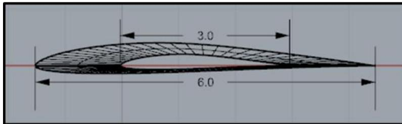
Figure 10: Cross-section of the final design, showing the cambered section shape and the taper from the middle to the tip.
