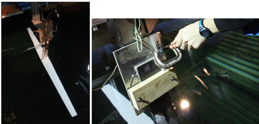
Figures 14 and 15: Towing configuration for the lift and drag tests done on the main foil (left). The bracket used to fix angle of attack is shown on the right.
