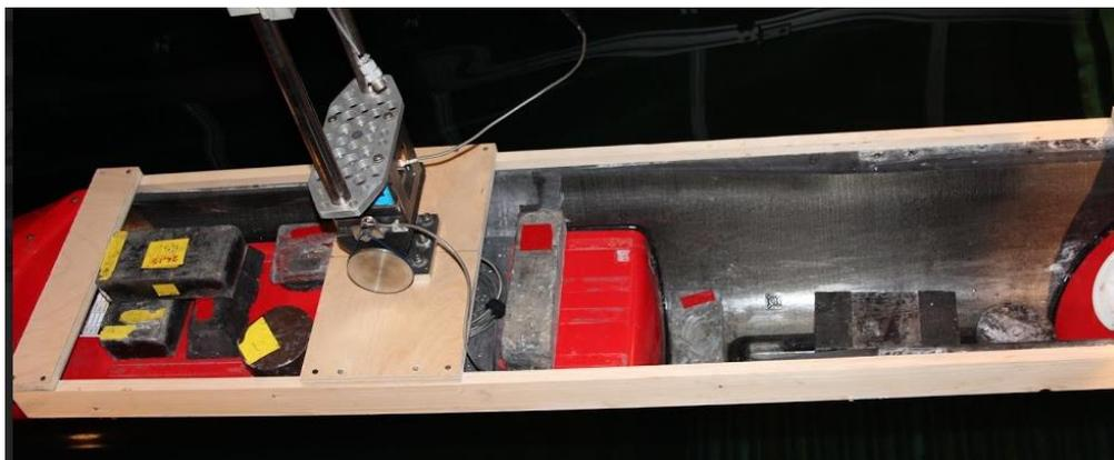
Figure 12: Test rig for the hull resistance tests. Resistance was measured using a 4-inch block gage.
