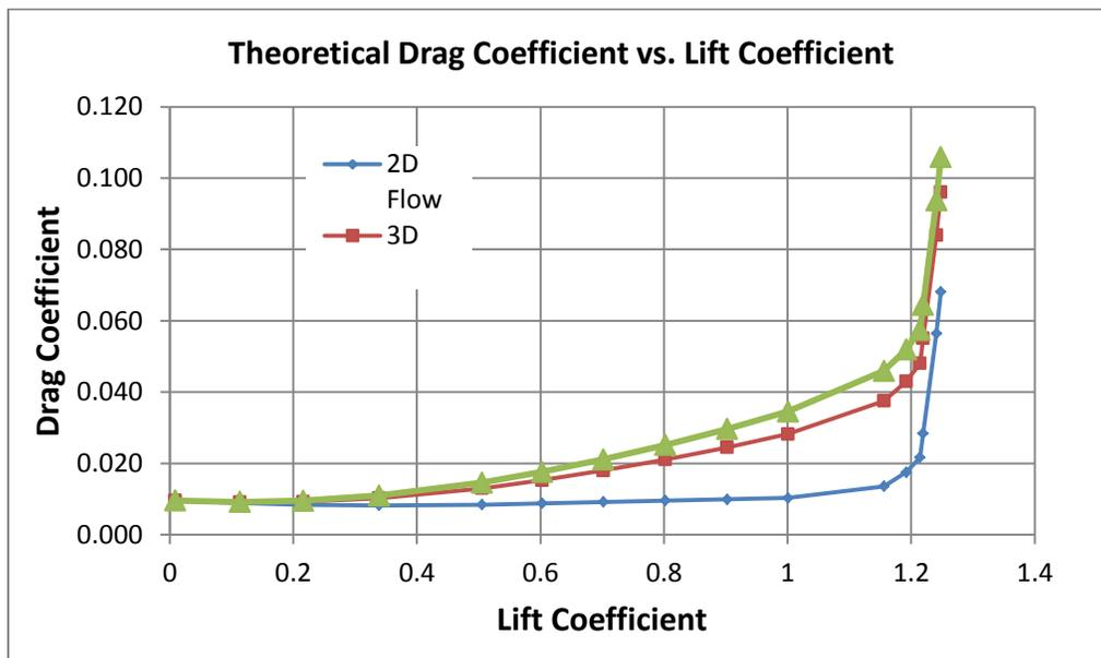
Figure 7: Adjustments to drag coefficient from 2D theoretical flow to 3D finitely submerged flow for the main foil.
