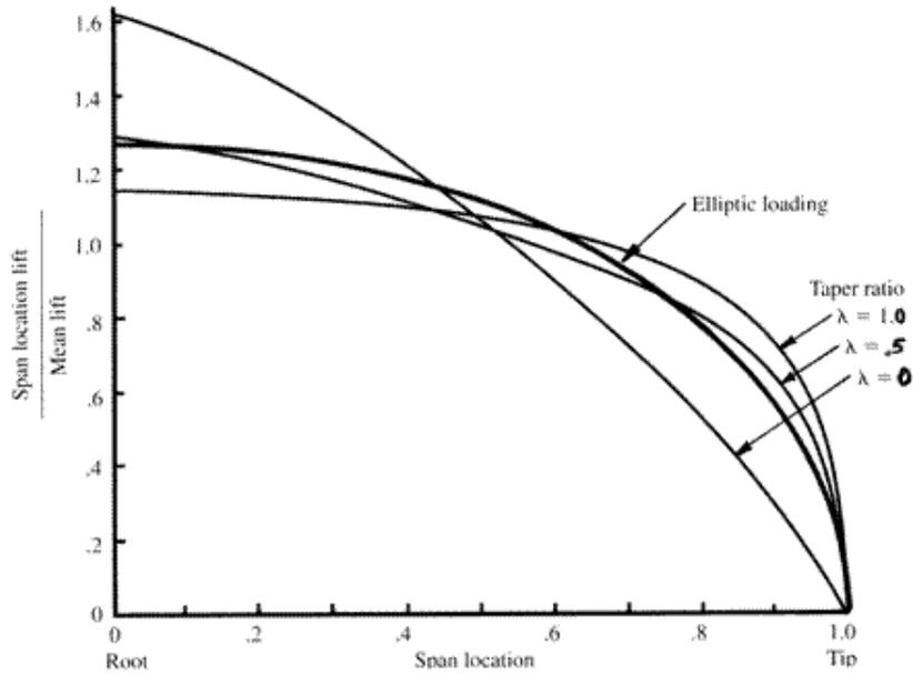
Figure 9: Typical lift distribution across different foil shapes
