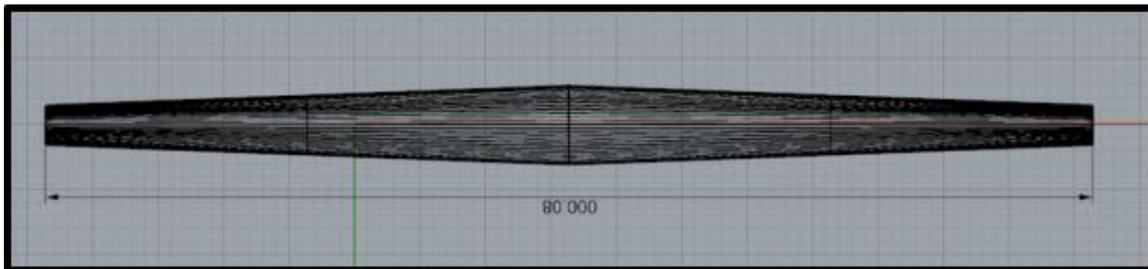
Figure 11: Top view of the main foil final design. Shows full 80-inch span.
