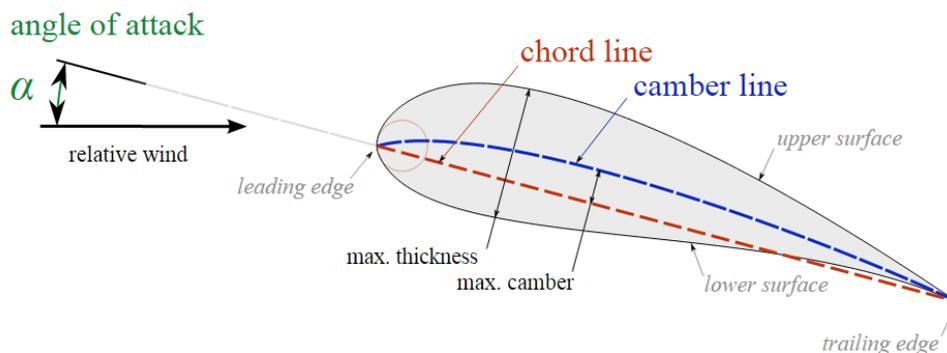
Figure 5: Cross-section of a typical cambered foil
