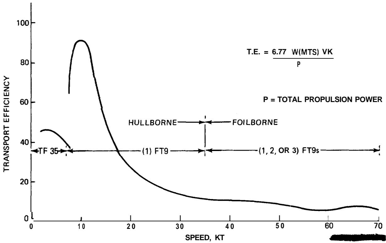
Fig. 2-18 Transport Efficiency vs Speed, Smooth Water (U)
