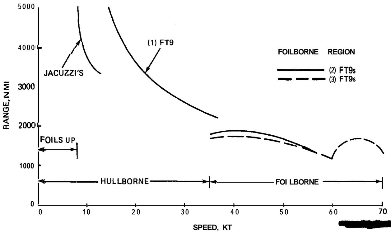
Fig. 2-21 Range vs Speed, No Ship Service Load (U)
