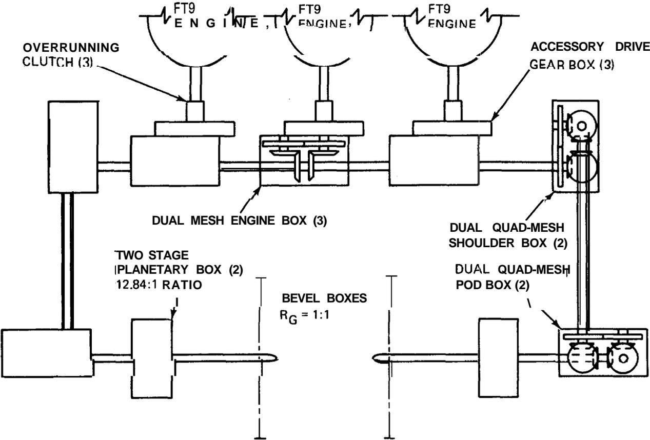
Fig. 2-34 Dual-Mesh/Dual-Quad Mesh Transmission System
