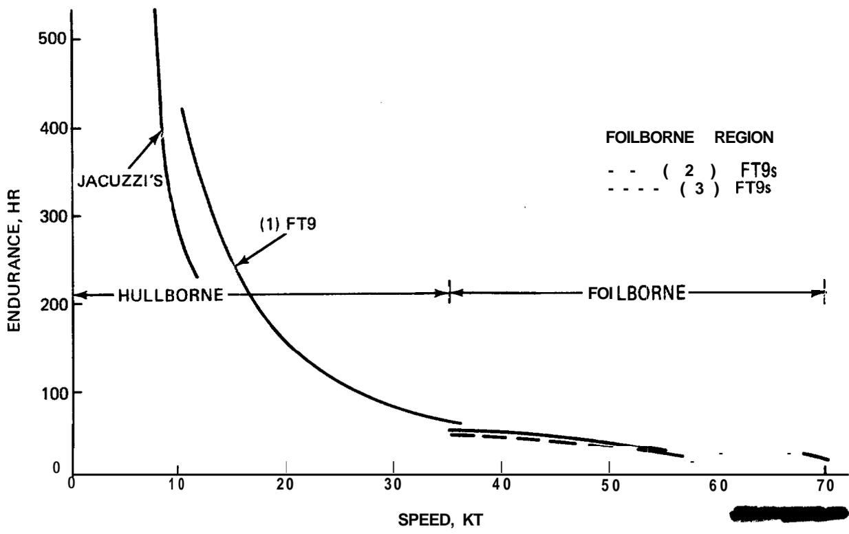
Fig. 2-24 Endurance vs Speed. Ship Service Load = .35 Mt/Hr (U)
