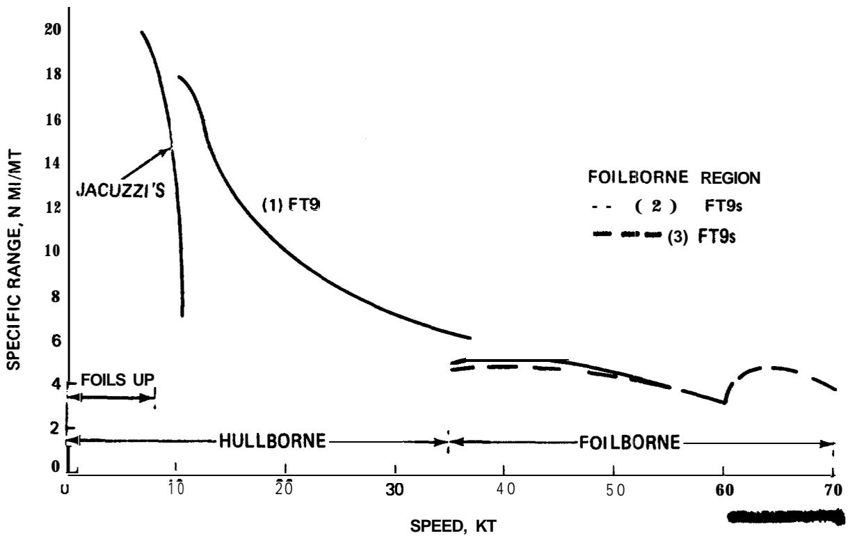
Fig. 2-19 Specific Range vs Speed, No Ship Service Load (U)
