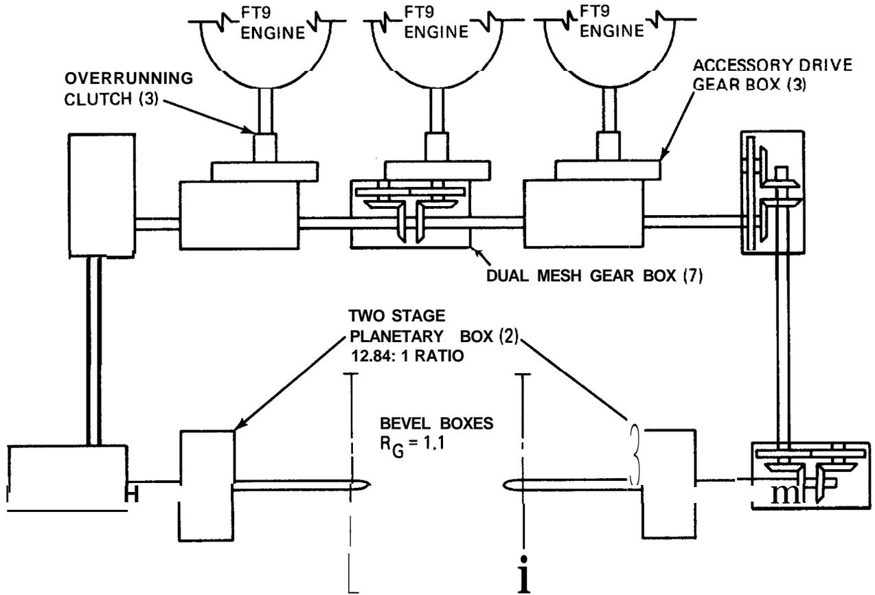
Fig. 2-33 Dual-Mesh Transmission System
