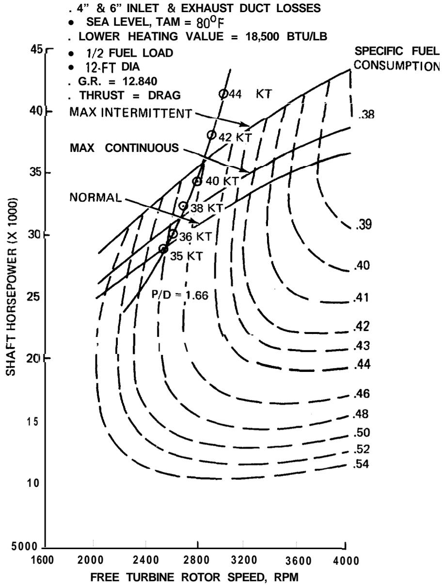
Fig. 2-28 FT9 Estimated Performance Characteristics, Foilborne One Engine and Two Propellers
