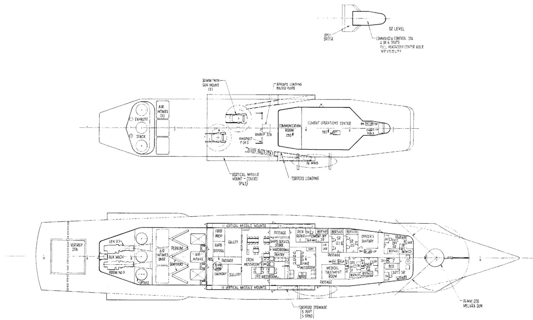
Fig. 2-3 Main Deck, 01 and 02 Levels, General Arrangement
