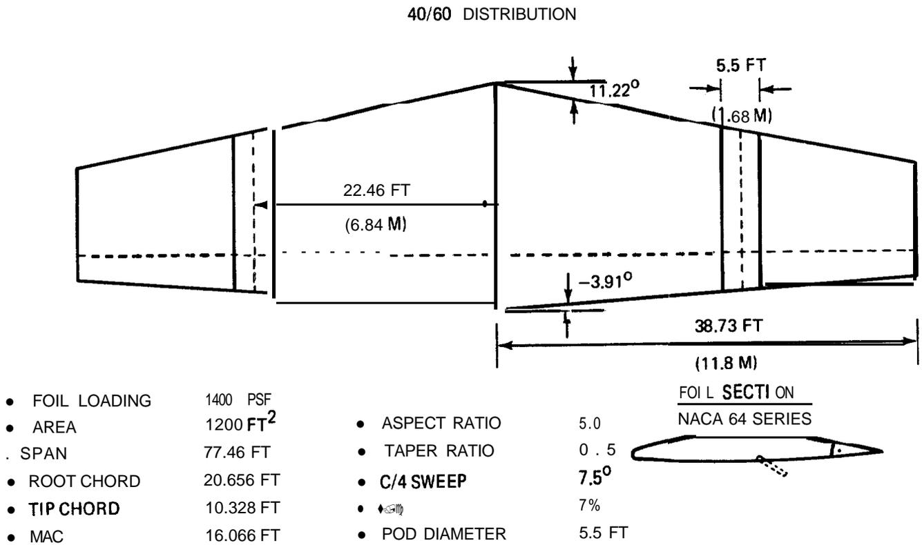
Fig. 2-36 Aft Foil Geometry
