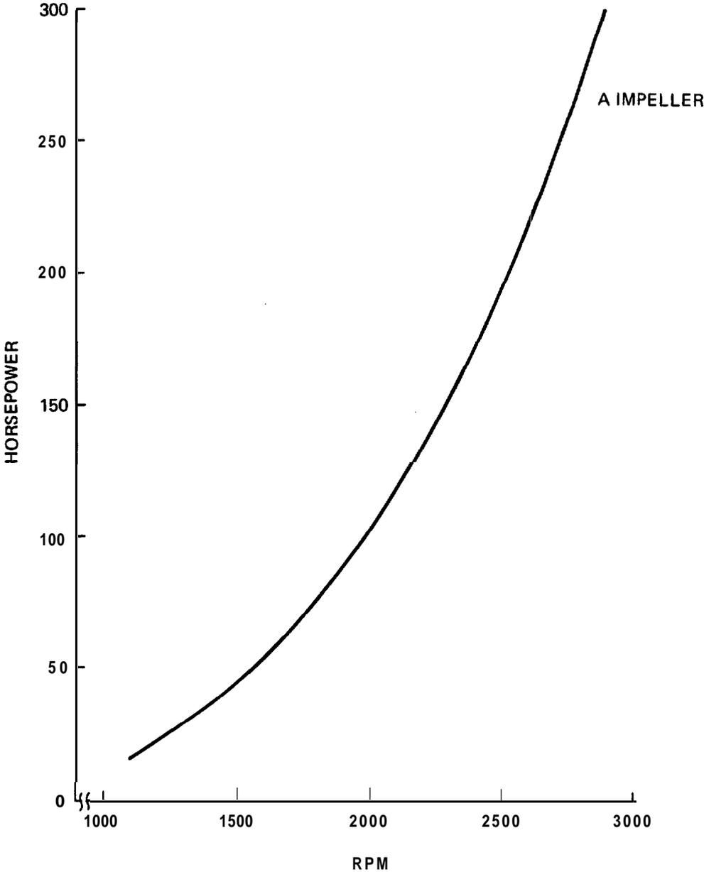
Fig. 2-30 Jacuzzi Jet 14YJ Power and RPM Characteristics
