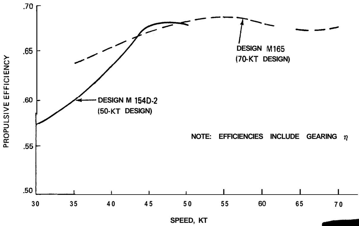
Fig. 3-2 Propulsive Efficiency Comparison (U)
