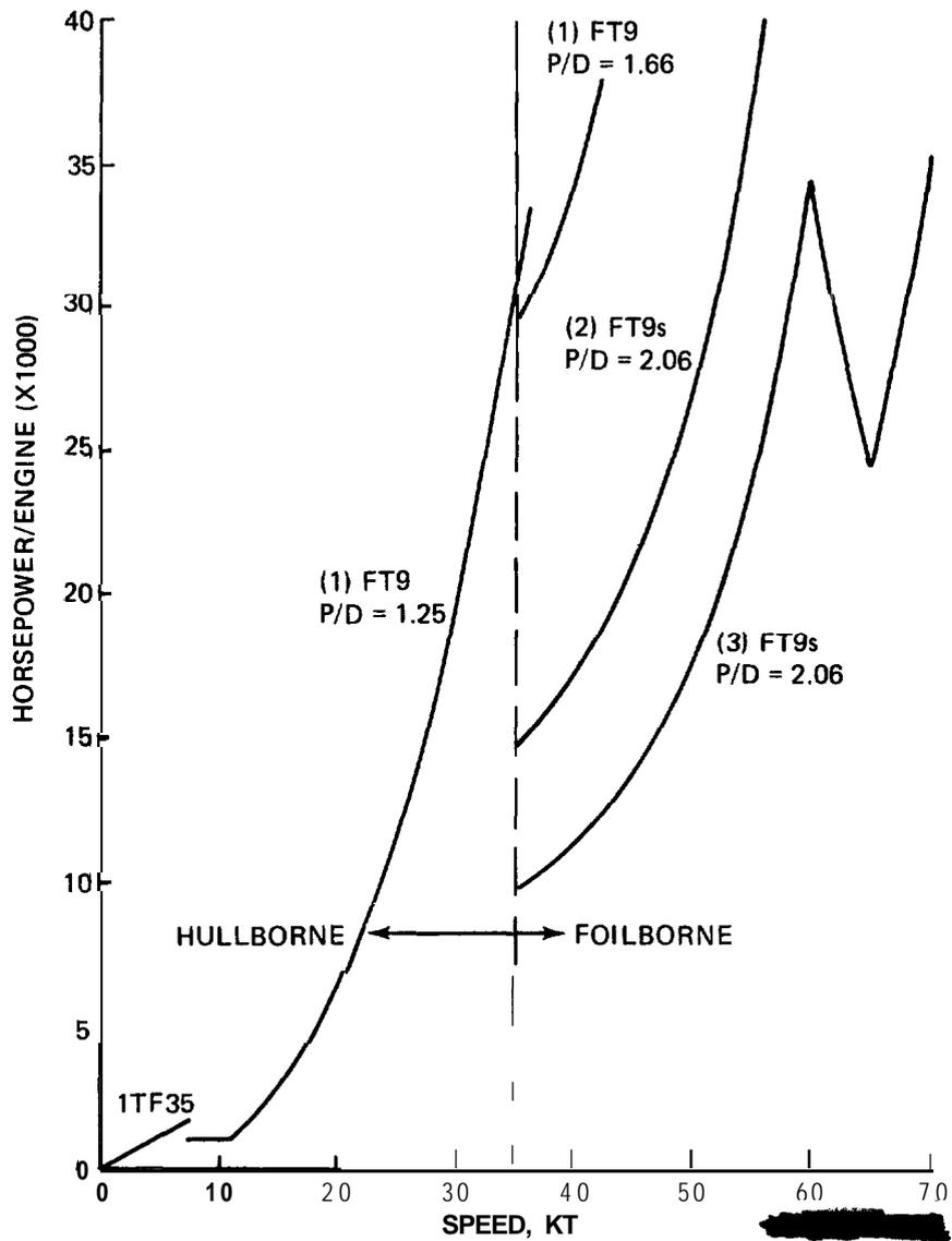
Fig. 2-15 Horsepower/Engine vs Ship Speed (U)
