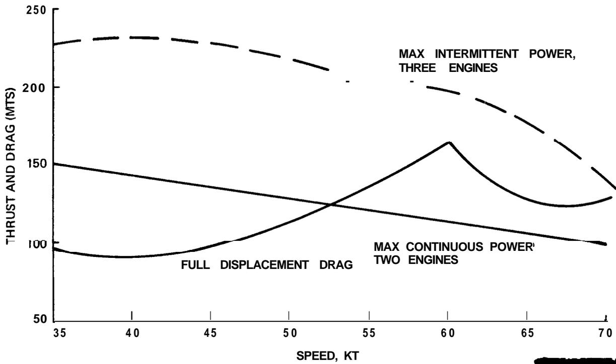
Fig. 2-13 Thrust and Drag vs Speed (U)
