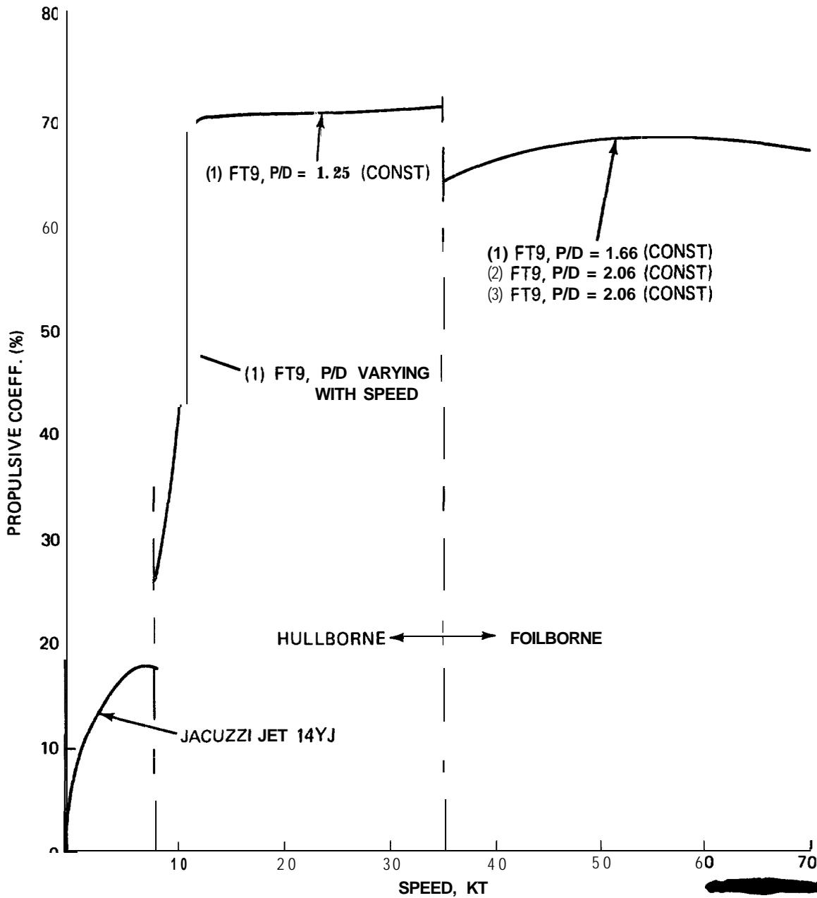
Fig. 2-16 Propulsion Coefficient vs Ship Speed (U)
