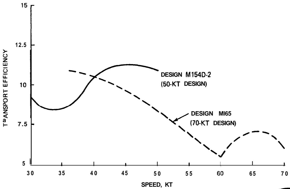
Fig. 3-4 Transport Efficiency Comparison (U)
