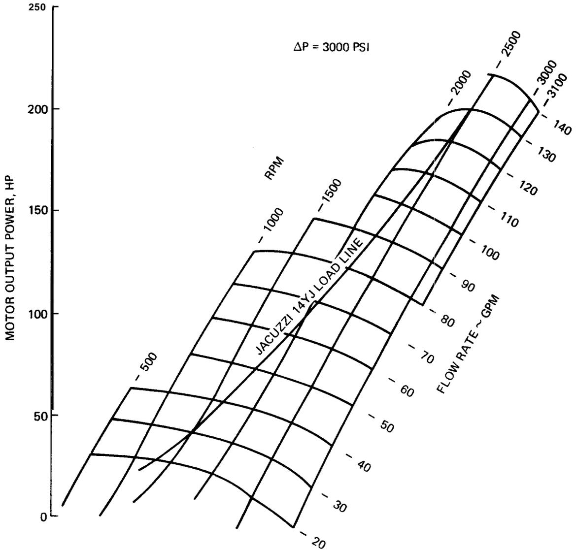
Fig. 2-29 Trimot A6V Hydraulic Motor Characteristics
