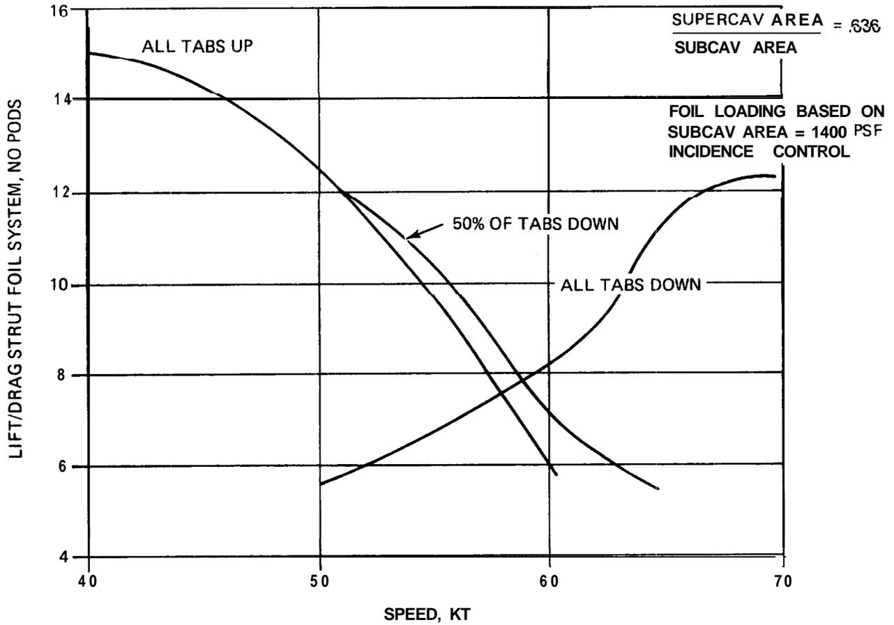
Fig. 2-8 Strut and Foil L/D, Incidence Control
