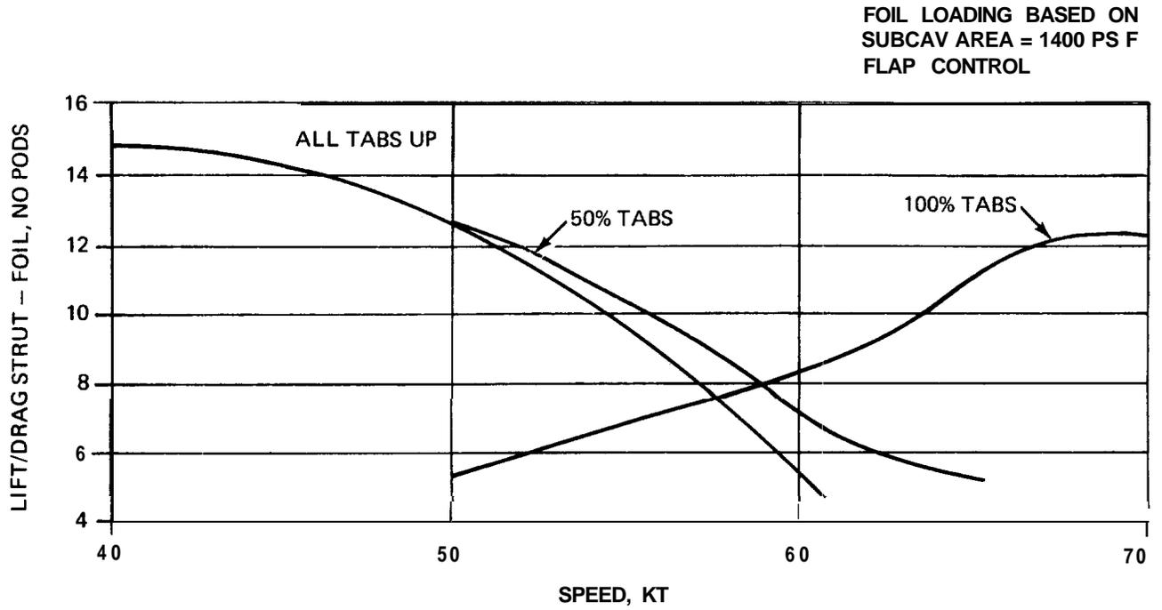
Fig. 2-9 Strut and Foil L/D, Flap Control
