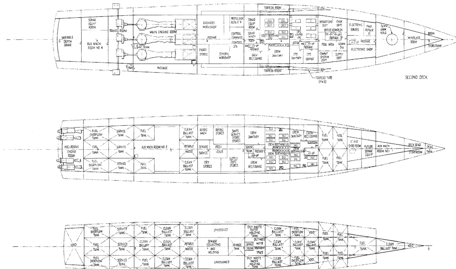
Fig. 2-4 Second Deck, First Platform and Hold, General Arrangement
