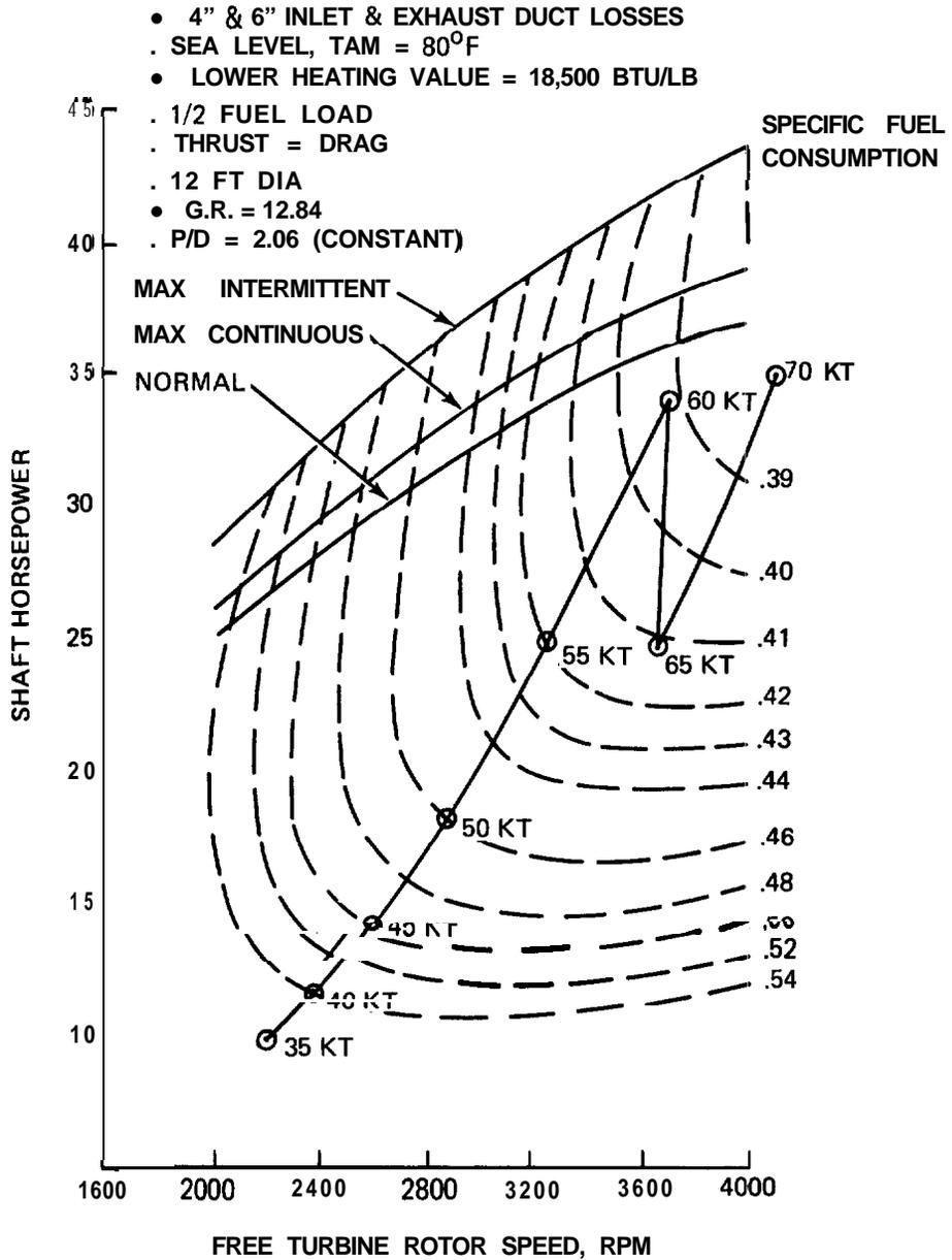
Fig. 2-26 FT9 Estimated Performance Characteristics, Foilborne, Three Engines and Two Propellers
