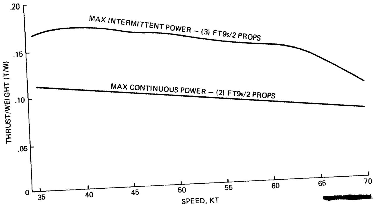
Fig. 2-14 Thrust/Weight vs Speed (U)
