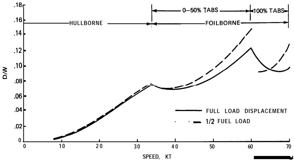
Fig. 2-12 Drag/Weight vs Speed (U)
