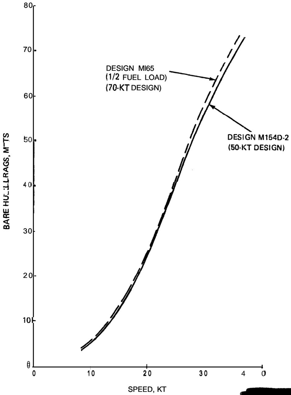
Fig. 3-1 Bare Hull Drag Comparison (U)
