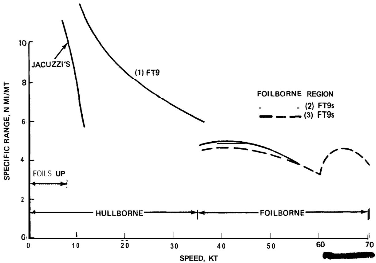
Fig. 2-20 Specific Range vs Speed, Ship Service Load = .35 Mt/Hr (U)
