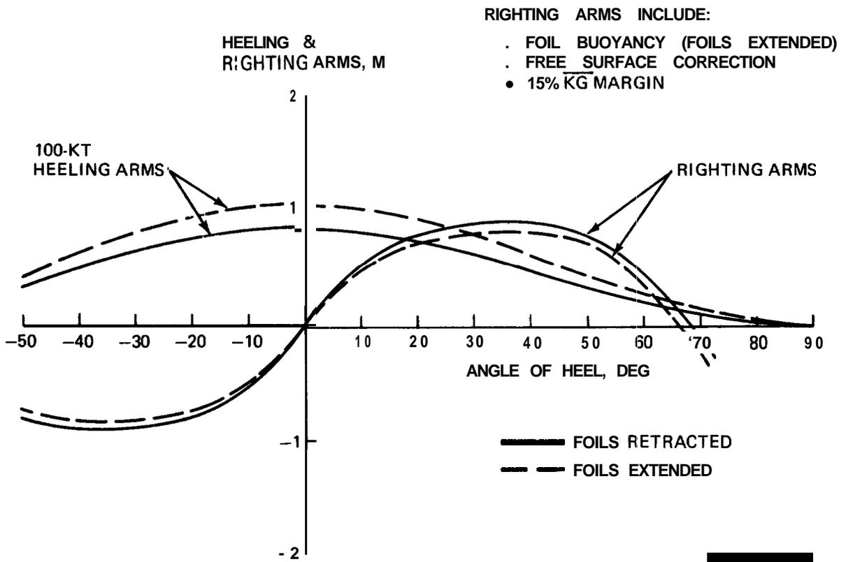
Fig. 2-25. Intact Stability, Burned Out Condition (U)
