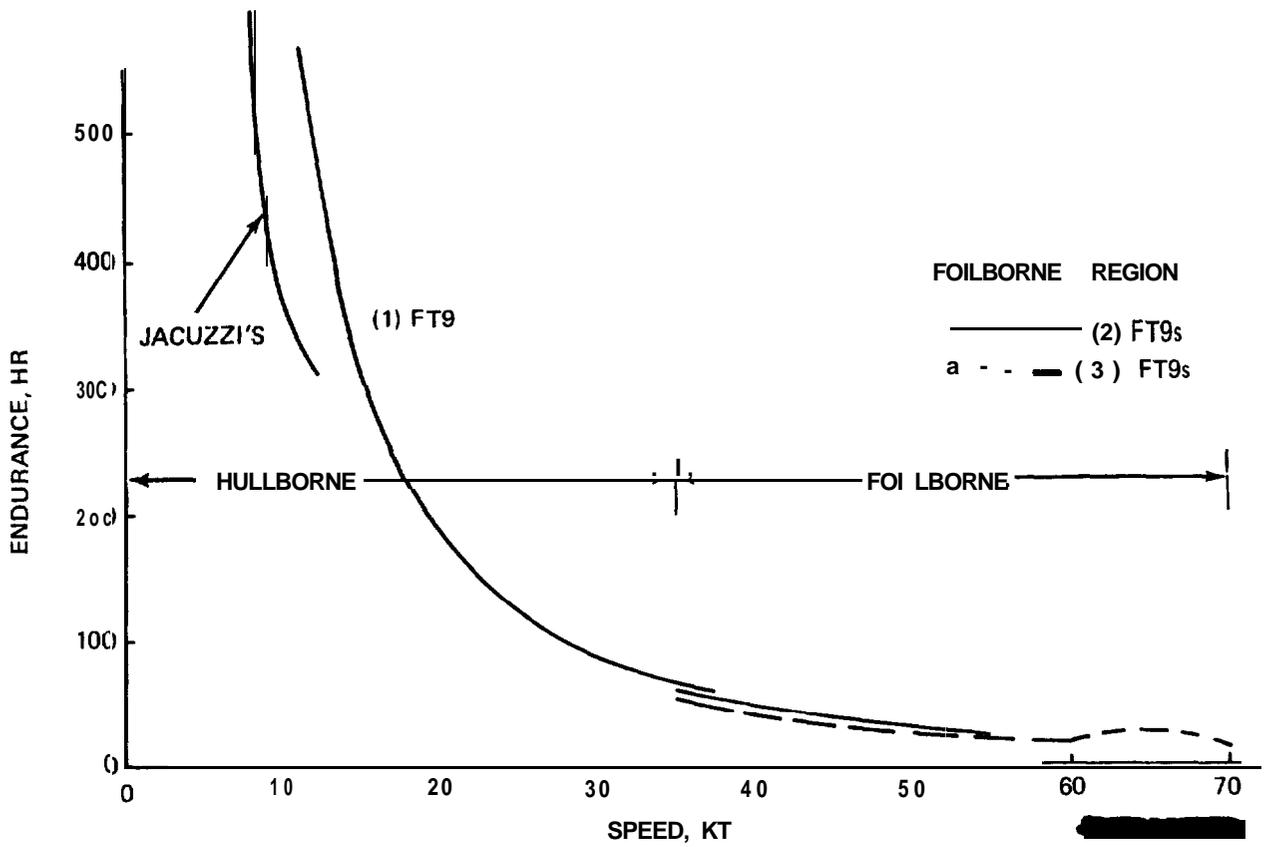
Fig. 2-23 Endurance vs Speed, No Ship Service Load (U)
