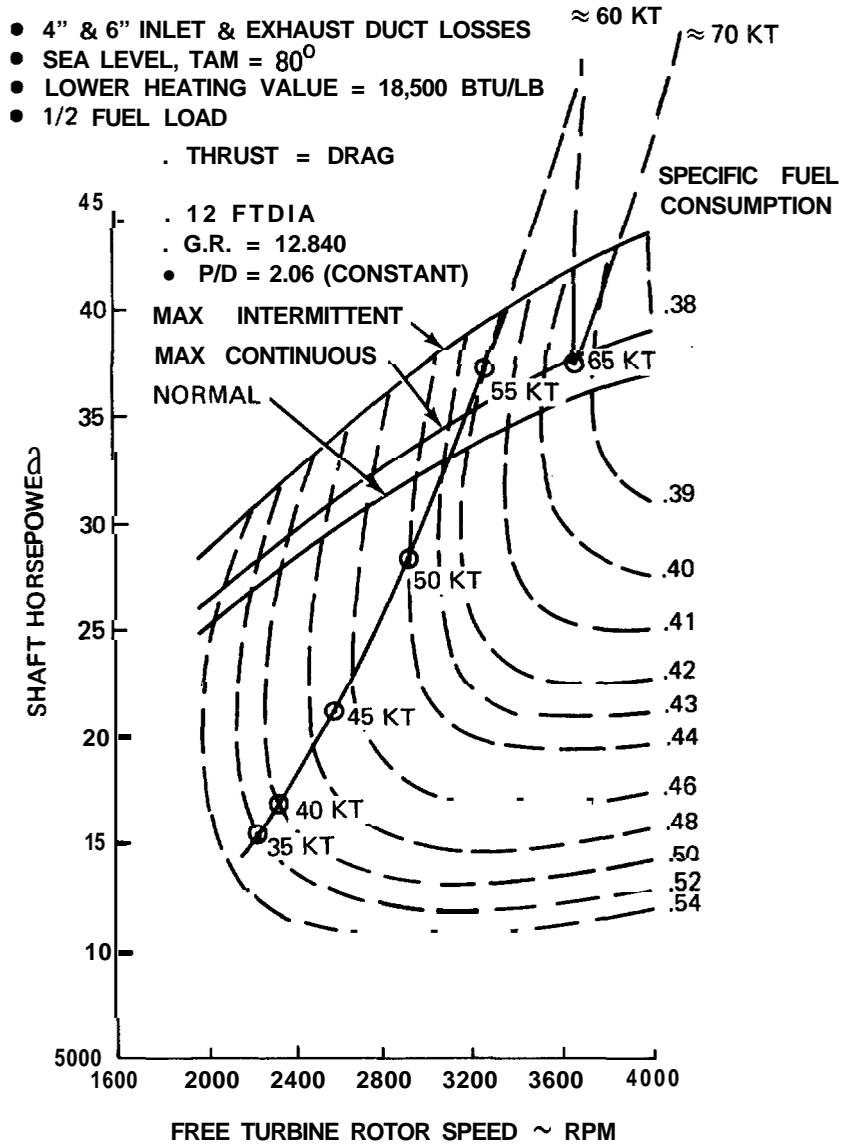
Fig. 2-27 FT9 Estimated Performance Characteristics, Foilborne, Two Engines and Two Propellers
