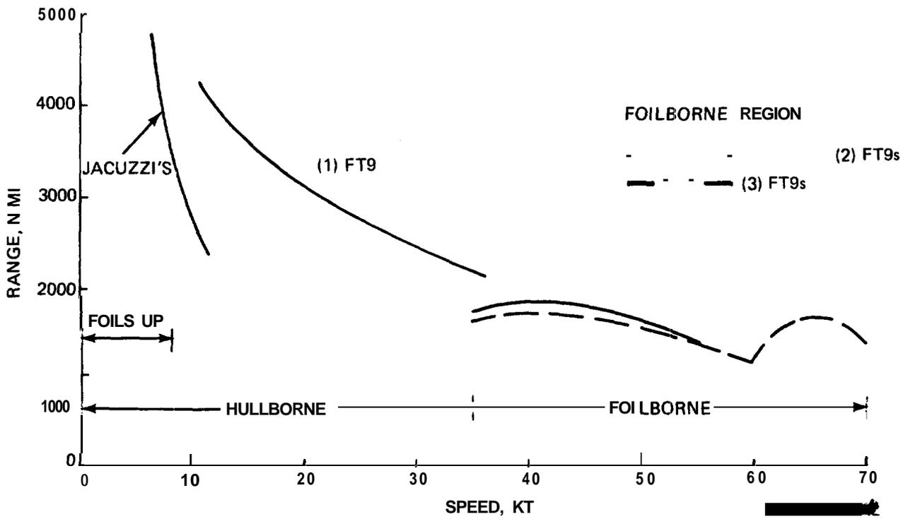
Fig. 2-22 Range vs Speed, Ship Service Load = .35 Mt/Hr (U)
