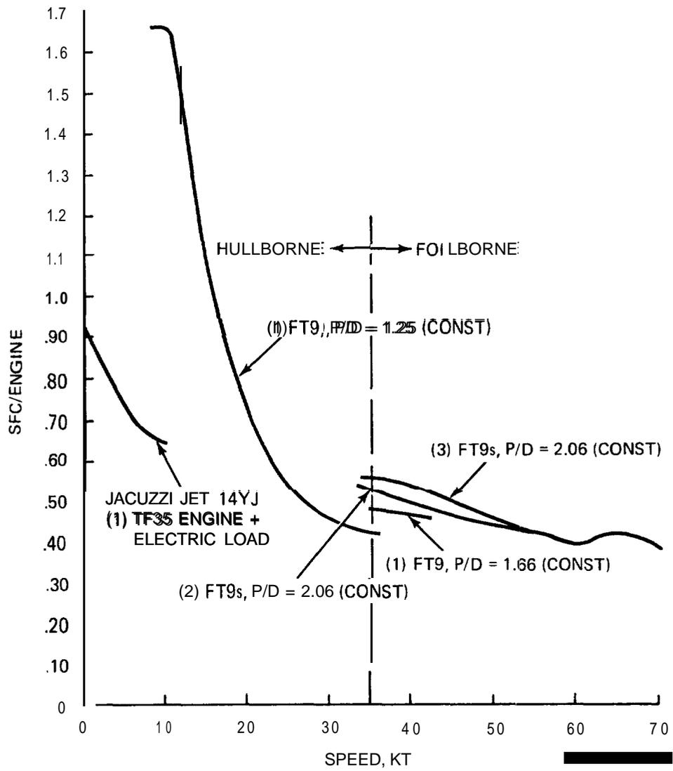
Fig. 2-17 SFC vs Ship Speed (U)
