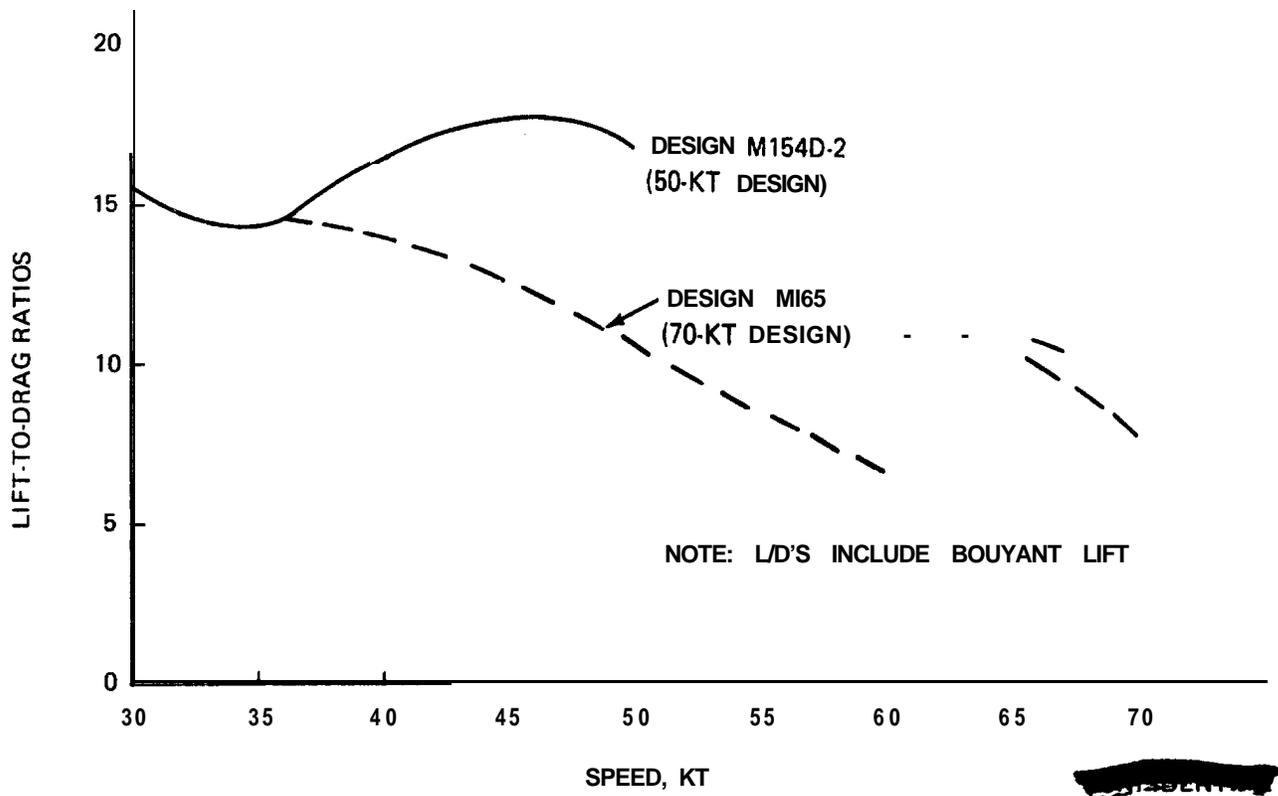
Fig. 3-3 Lift-to Drag Ratio Comparison (Foilborne) (U)
