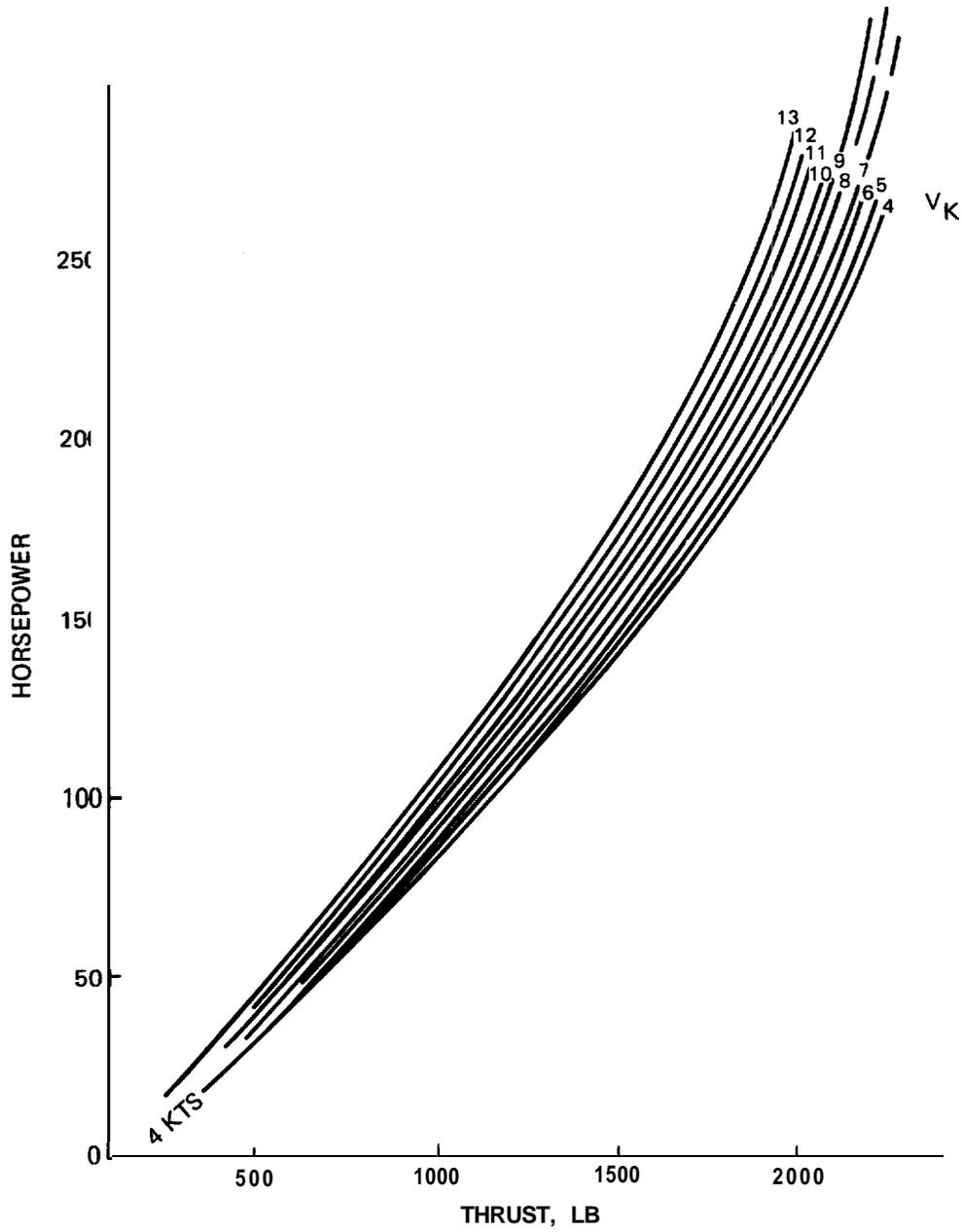
Fig. 2-31 Jacuzzi Jet 14YJ Thrust Characteristics
