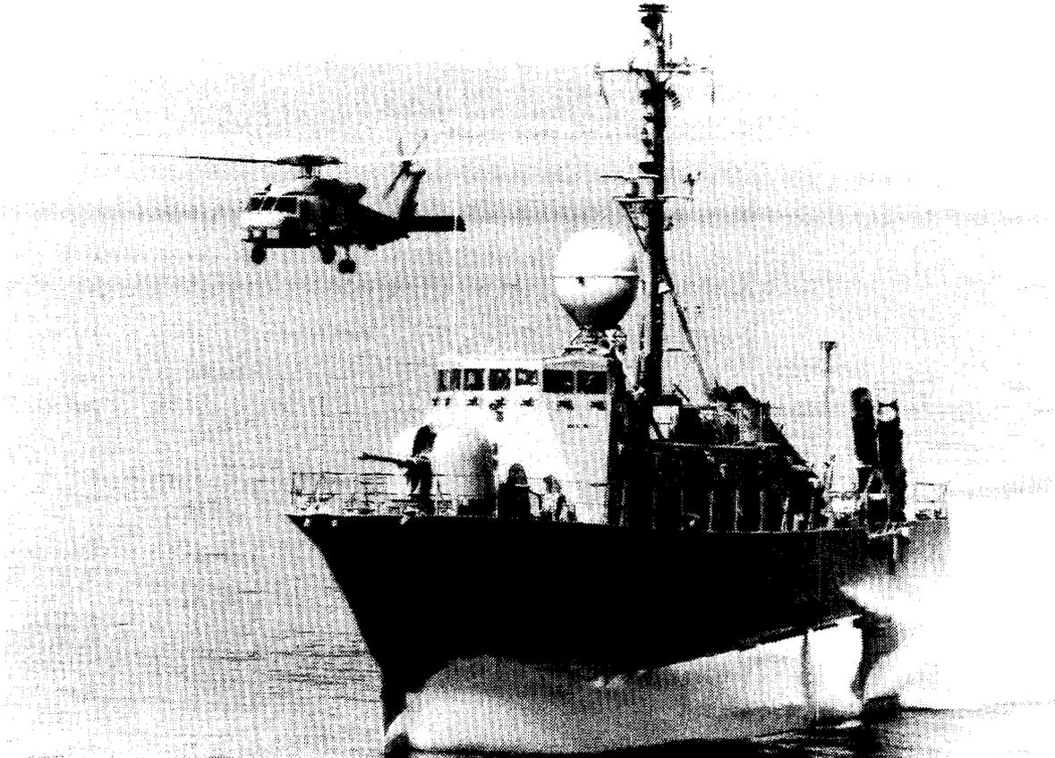
USS PEGASUS (PHM 1) was launched on 09 November 1974, in Seattle, Washington as the lead ship in a new class of U.S. Navy hydrofoil. PEGASUS proved the utility of hydrofoil technology in a combatant application, and did so effectively during her 19 years of service.
