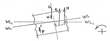
When the ship trims, the center of buoyancy will move but the center of foil lift will remain stationary.
