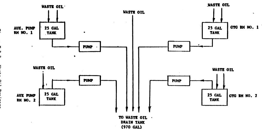
Figure E.2-3. Waste Oil Drainage
