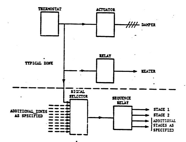
Figure E.3-1. Functional Block Diagram for HVAC Control System
