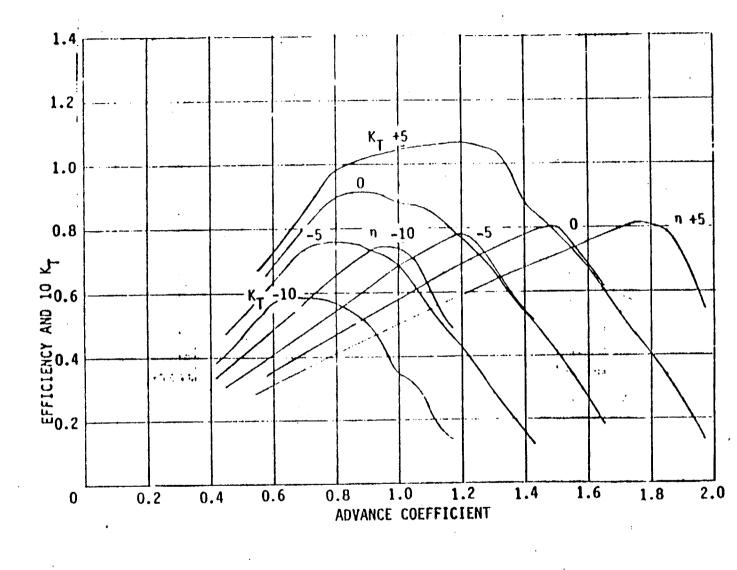
Figure 2-5 MDC 1500 PROPELLER (50 PERCENT SUBMERGED)
