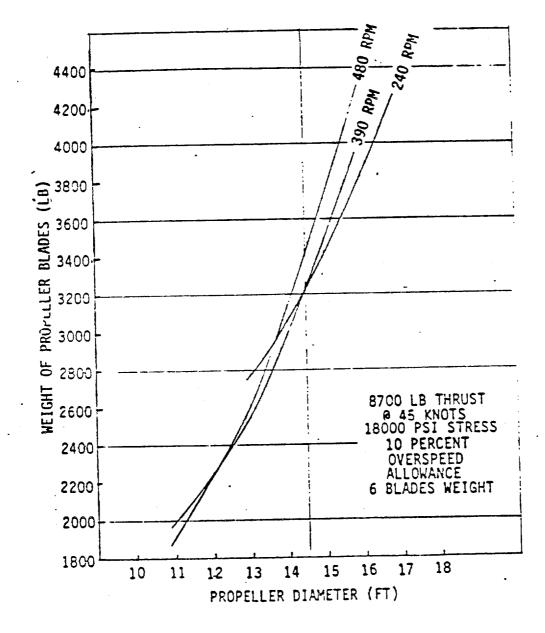
Figure 2-3 BLADE WEIGHT VERSUS SIZE
