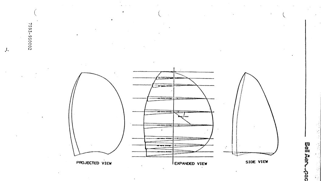
Figure 1-4 PROPELLER BLADE SECTIONS EXPANDED VIEW
