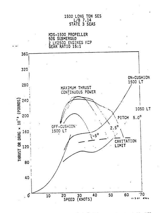
Figure 2-7 MAXIMUM THRUST ON CUSHION - LM2500 ENGINES, MCP
