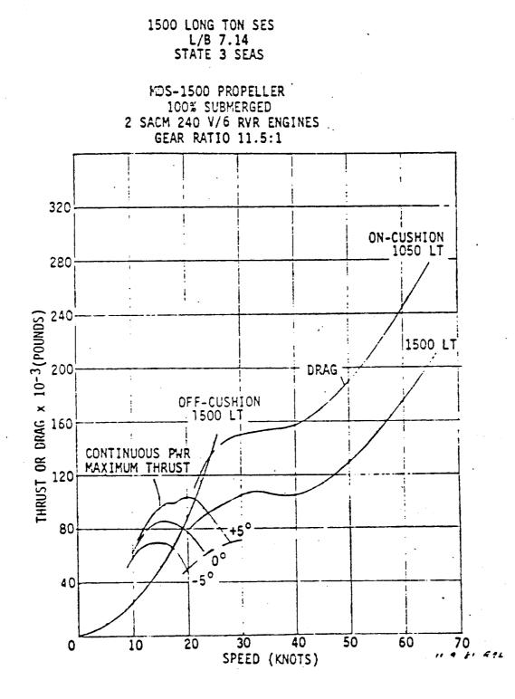
Figure 2-9 MAXIMUM THRUST OFF CUSHION - SACM ENGINES
