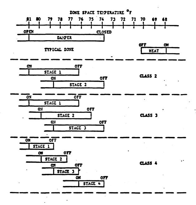
Figure E.3-2. Compressor Staging Concept
