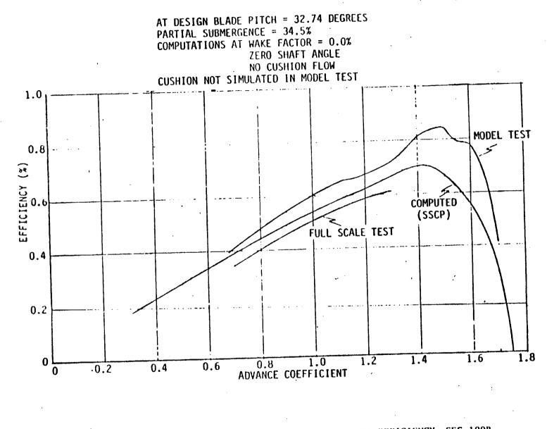
Figure 1-1 COMPUTED AND TEST PROPELLER EFFICIENCY SES-100B
