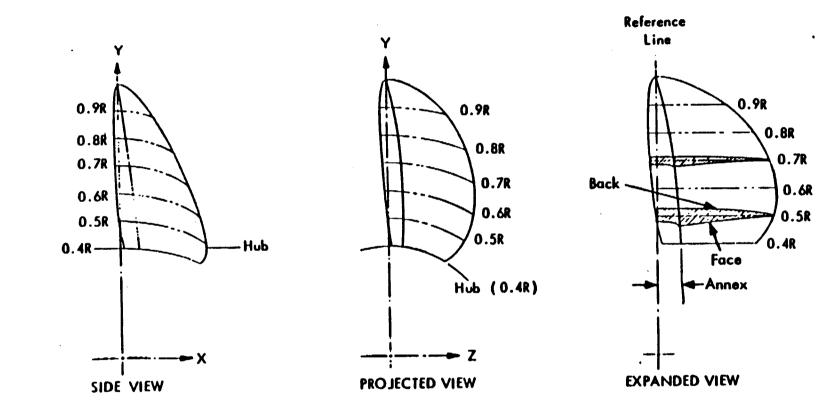
Figure B.l. Ventilated Propeller Shapes and Sections
