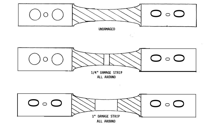
FIGURE 2 COATING CONFIGURATION
