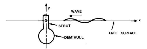
Figure 1 - Coordinate System Used in SWATH Section Study
