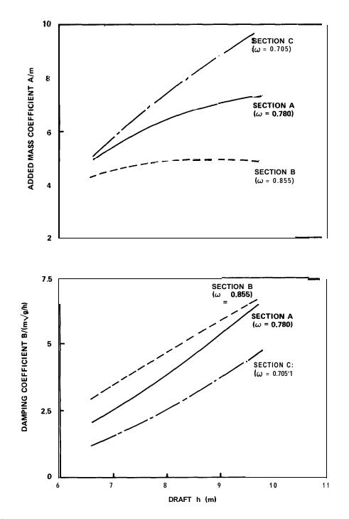
Figure 5 - Added Mass and Damping Coefficients of SWATH Sections for Heave Resonance as a Function of Draft
