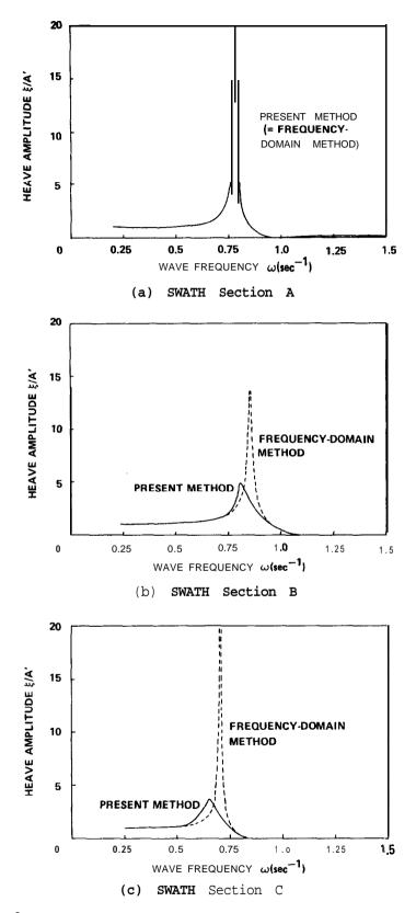
Figure 3 - Heave Motion of the Three SWATH Sections Studied
