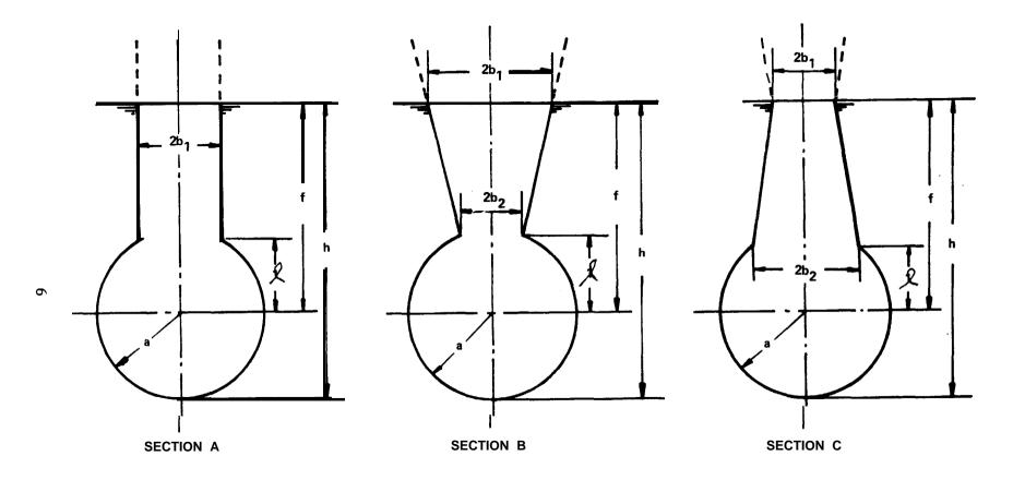
Figure 2 - SWATH Sections Chosen for Two-Dimensional Numerical Test
