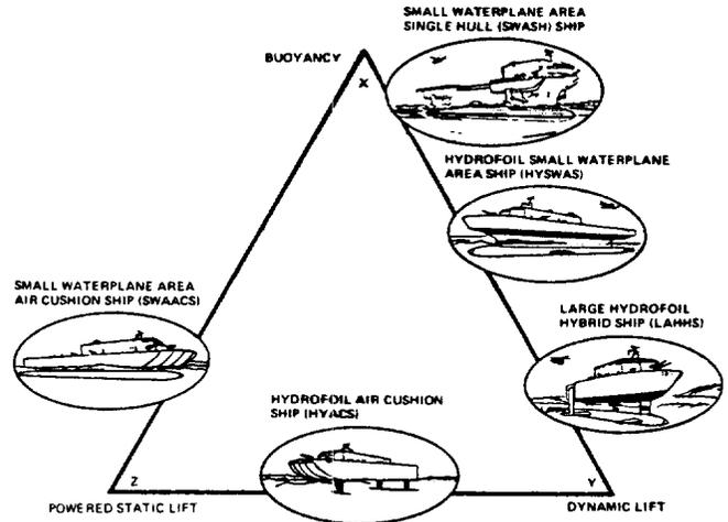
FIGURE 1 - SUSTENTATION TRIANGLE WITH HYBRID CONCEPTS
