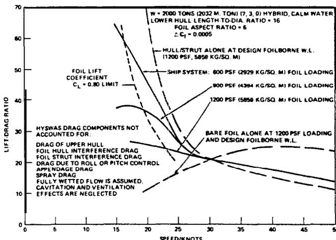
FIGURE 4 - HYSWAS LIFT-DRAGE RATIO
