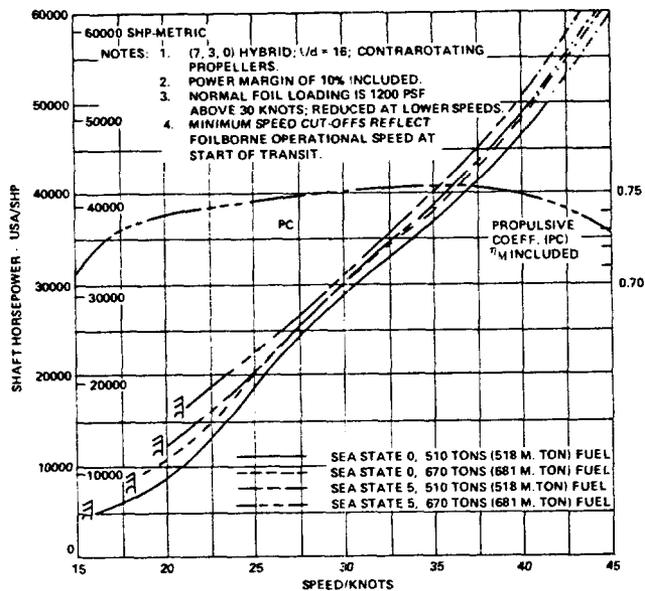
FIGURE 5 - SPEED POWER OF A 2000-TON HYSWAS
