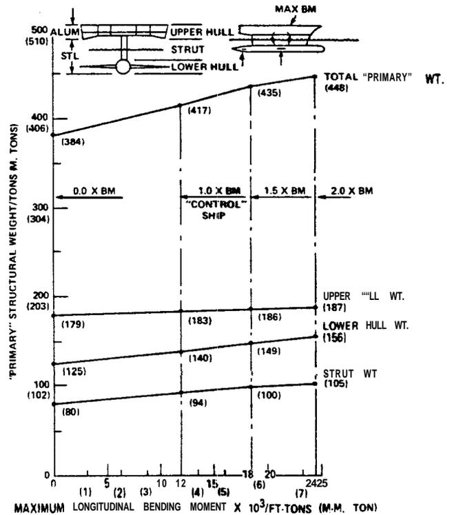
FIGURE 14 - "PRIMARY" STRUCTURAL WEIGHT VERSUS MAXIMUM LONGITUDINAL BENDING MOMENTS (12)
