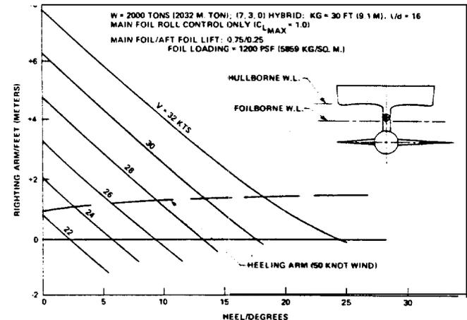
FIGURE 9 - HYSWAS FOILBORNE RIGHTING ARM CHARACTERISTICS; FOIL LOADING = 1200 PSF (5859 KG/SQ. M)
