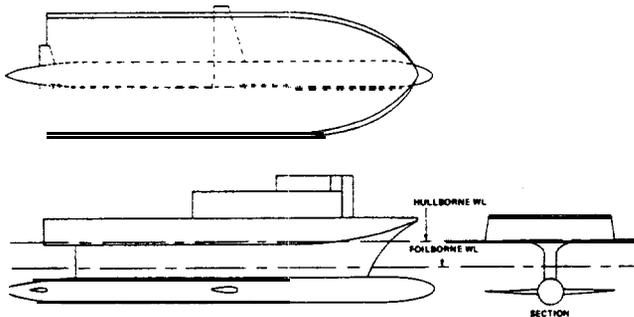
FIGURE 2 - SKETCH OF THE HYDROFOIL SMALL WATERPLANE AREA SHIP (HYSWAS) FORM.
