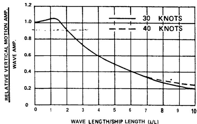
FIGURE 12 - 2000-TON HYSWAS RELATIVE VERTICAL MOTION OF FORWARD END OF STRUT IN REGULAR HEAD WAVES WITH CONTROLS FIXED
