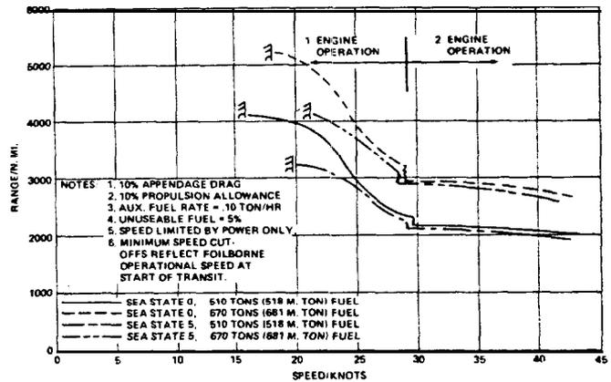
FIGURE G - ESTIMATED RANGE OF A 2000-TON HYSWAS: PAYLOAD = 177 TONS (180 M. TON)
