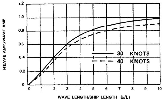
FIGURE 11 - 2000-TON HYSWAS HEAVE MOTION IN REGULAR HEAD WAVES WITH CONTROLS FIXED
