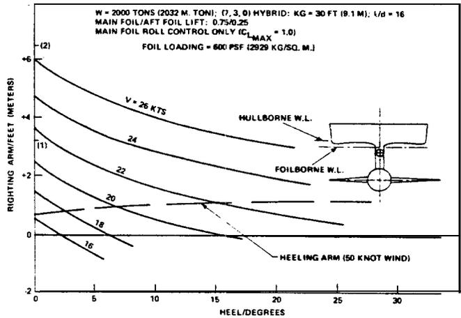
FIGURE 8 - HYSWAS FOILBORNE RIGHTING ARM CHARACTERISTICS; FOIL LOADING, = 600 PSF (2929 KG/SQ. M)
