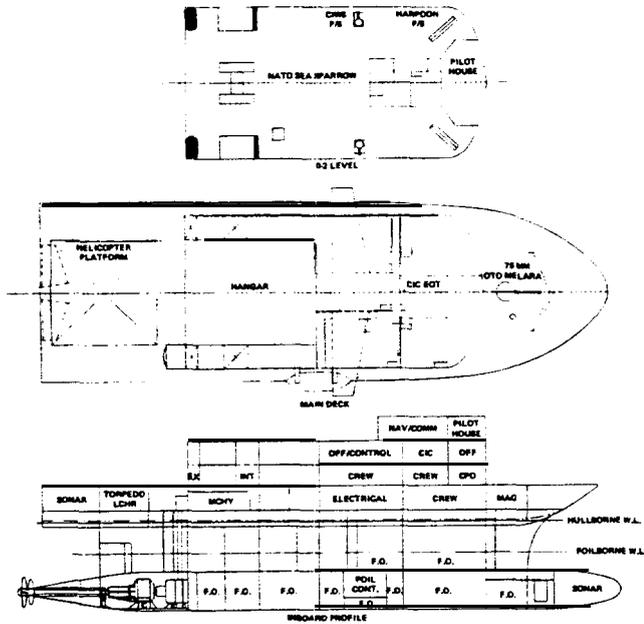
FIGURE 19 - 2000-TON HYSWAS COMBATANT ARRANGEMENT
