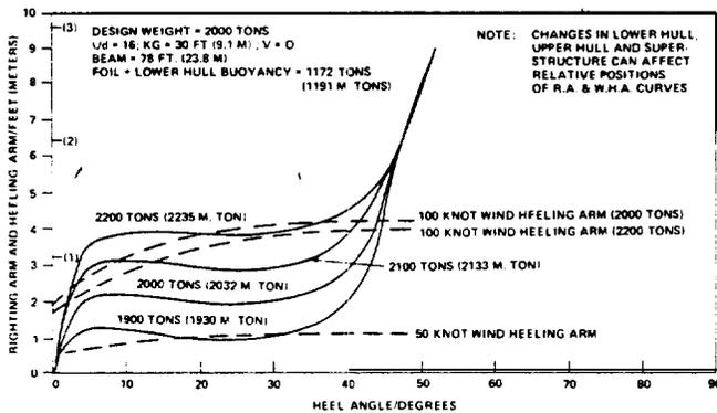
FIGURE 7 - HYSWAS HULLBORNE INTACT STABILITY CHARACTERISTICS
