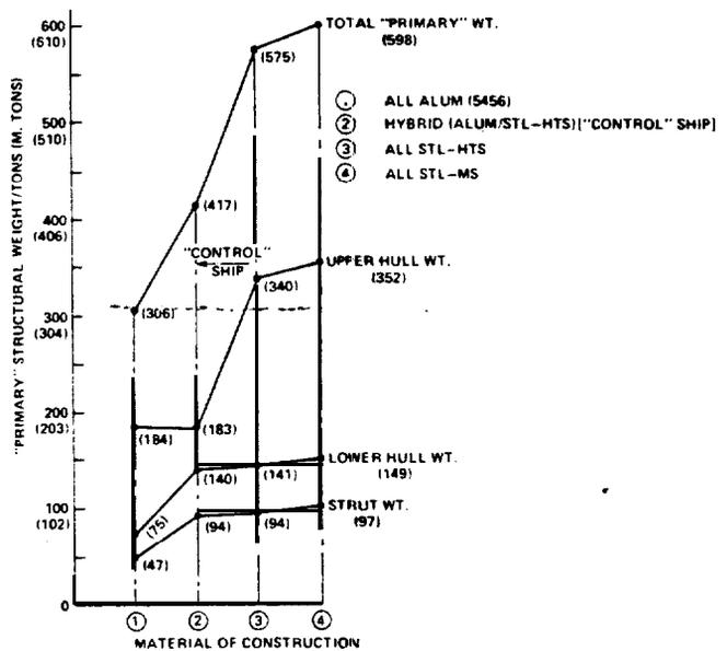
FIGURE 15 - "PRIMARY" STRUCTURAL WEIGHT VERSUS MATERIAL OF CONSTRUCTION (12)
