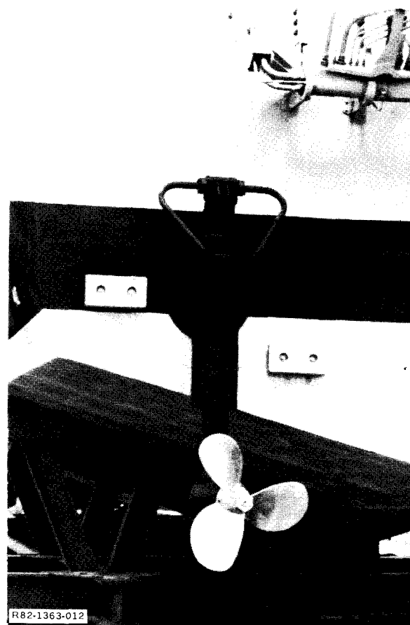
Fig. 14 Hydraulically Driven Sterndrive Installed on SHIMRIT's Transom
