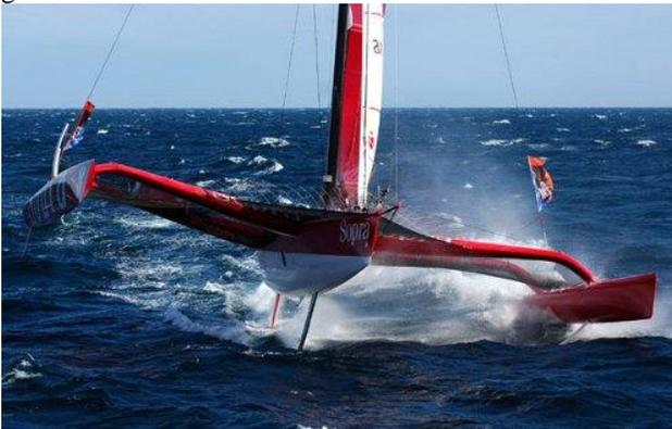
Figure 1. ORMA 60 with lifting foils
