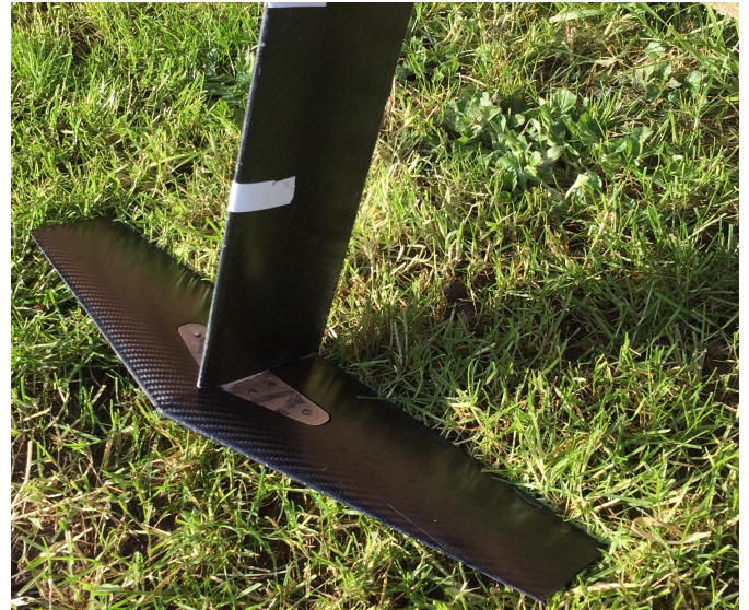
Figure 6: Elevator attachment for the rudder.
