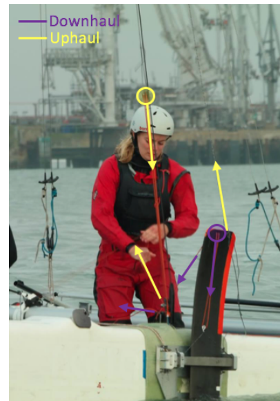
Figure 13: Up and downhaul control system.
