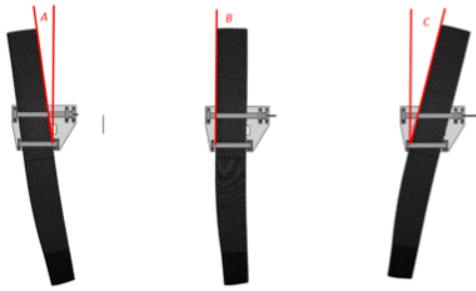
Figure 11: Final Designs rake angles. A = -8.4^\circ , B = 0^\circ , C = 13.7^\circ
