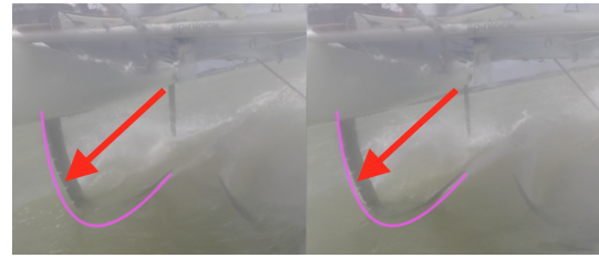
Figure 28: Frontal View of board movement as tip comes out of water during four point foiling.
