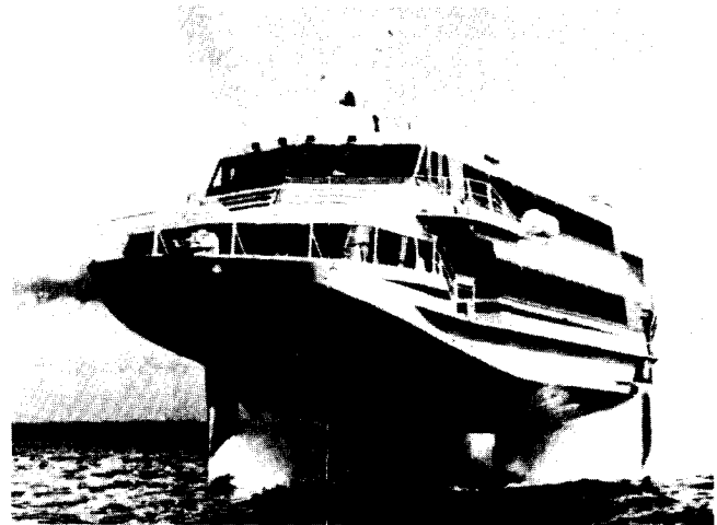
Figure 56. The only commercial hydrofoil built in the U.S. is the Boeing model 929 Jetfoil.
