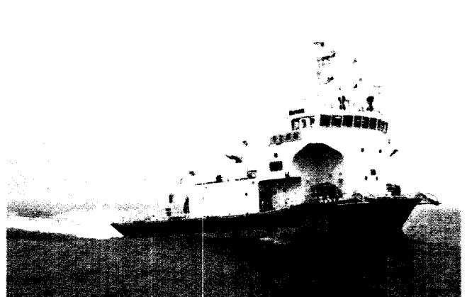
Figure 23. Ohtori, SWATH-Type Hydrographic Survey Vessel by Mitsubishi.
