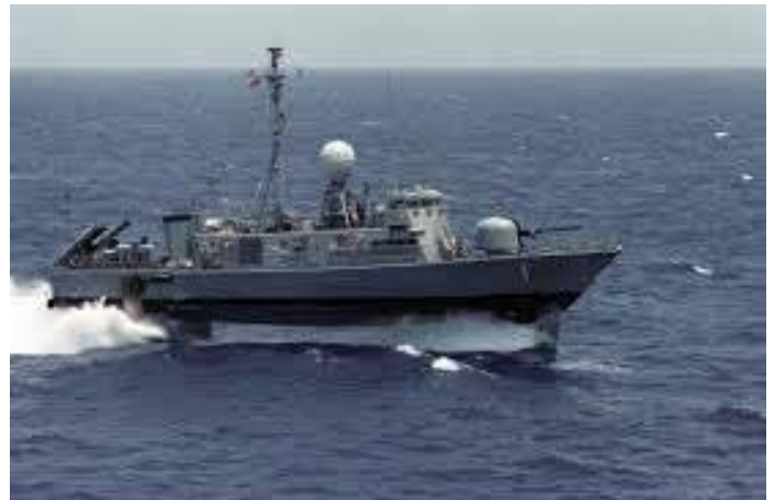
The Boeing developed and built hydrofoil missile boat USS Pegasus.
