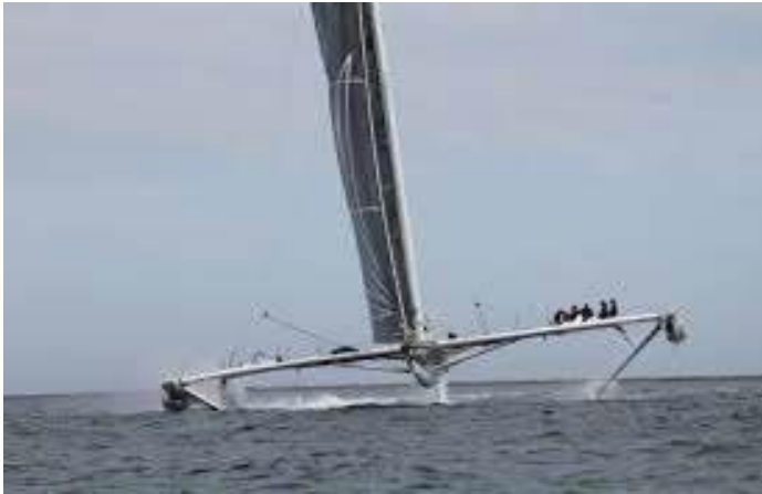
In 2009 the large foiling trimaran l'Hydroptere achieved 51 knots over a measured nautical mile. It actually exceeded 55 knots during the speed attempt.
