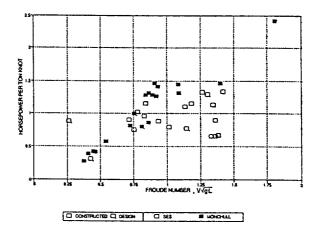
Figure 3-13. Installed Power/Full-Load Displacement/Speed Versus Froude Number
