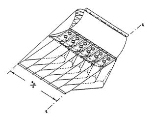
Figure 3-8. Illustration of Bag-and-Finger Bow Seal
