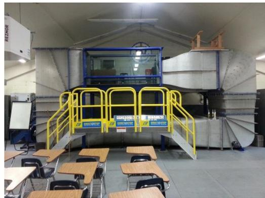
Figure 24. Haeberle Laboratory Flow Channel
