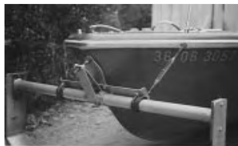
Fig. 4 — The bow foil is attached by four bolts. Note the angle adjustment plate and threaded rod positioned above the center of the cross tube.
