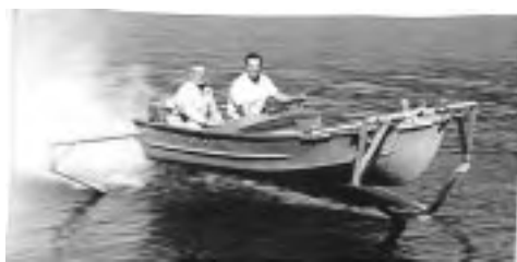
Fig. 2 — This 1954 three-Vee hydrofoil attained 35 mph with a 25 hp Johnson outboard. The author is driving, and his father is seated next to him.
