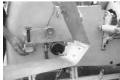
Fig. 8 — Each stern hydrofoil is mounted to the transom with three bolts, one of which is used to adjust its angle by rotating the large knurled knob. The small container with the black lid to the left of the inner end of the foil contains 500-ft of coiled cord for retrieving the foil if it hits an obstacle and shears free from its mount.
