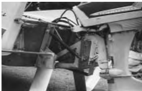
Fig. 5 — Each aft hydrofoil is bolted to the transom, and retracts about a 45-degree axis at the inboard end. Note the adjustable spring-loaded motor mount, and the short-shaft outboard.
