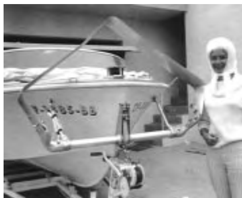
Fig. 7 — The bow foil can be retracted from the driver's seat, or adjusted in angle by the driver when underway.
