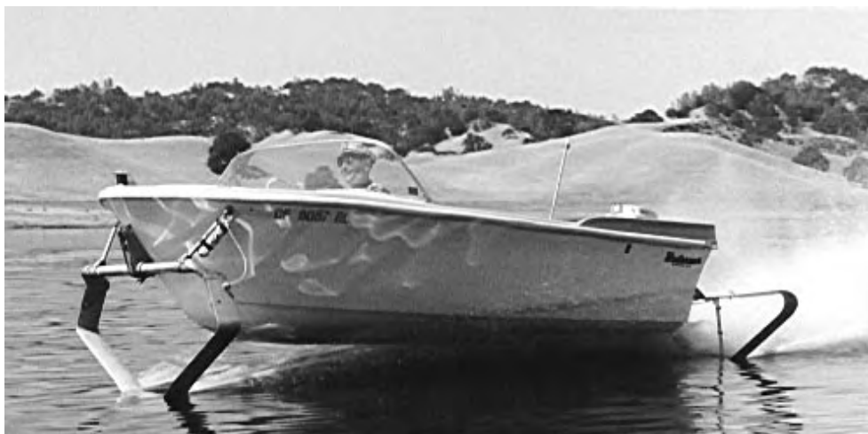
Fig. 9 — Boat equipped with the production Up-Right Hydrofoil Kit. This boat achieved 47 mph with a 65 hp Mercury outboard, and could carry six people.
