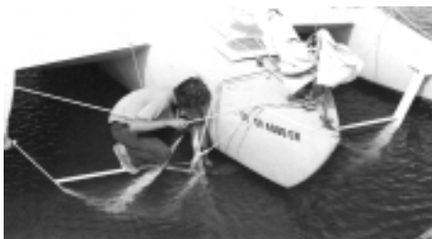
Setting the bow foil by inserting one of two shear bolts below the waterline. It is a wet job out at sea.
