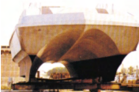
USA Catamarans' Super Critical Dyna-Cat Hull
