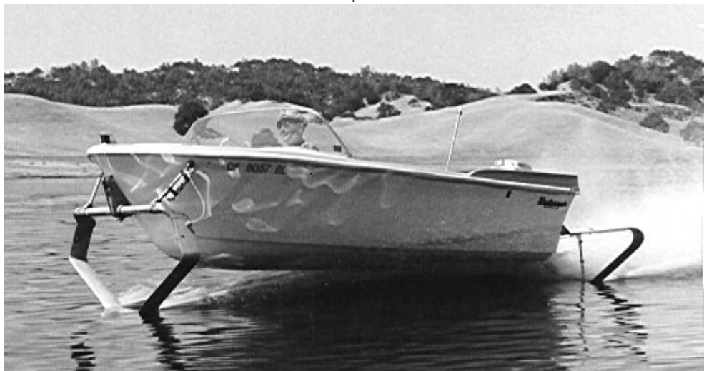
With the Upright Hydrofoil Kit installed, this boat achieved 47 mph with a 65 hp Mercury outboard motor.
