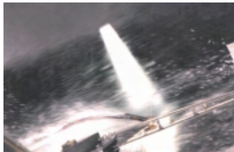
View over the bow with the bow foil submerged at 2 ft depth. Note the small twig caught on the strut.
