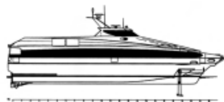
General arrangement of Morye 30m foil assisted catamaran
