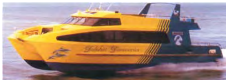
Teknikraft Design 18m foil assisted catamaran Discovery IV was delivered to Dolphin
