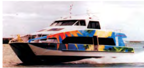
Lagilagi is the fourth foil assisted catamaran from Teknikraft Design and Q-West
