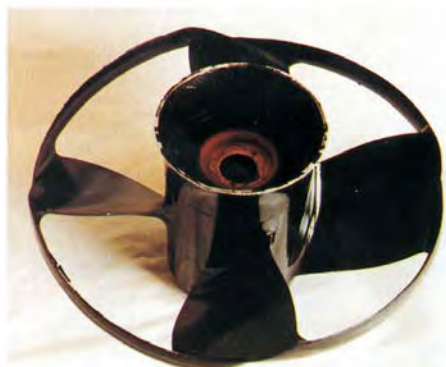
The RingProp configuration reportedly improves thrust and overall performance at all speeds
