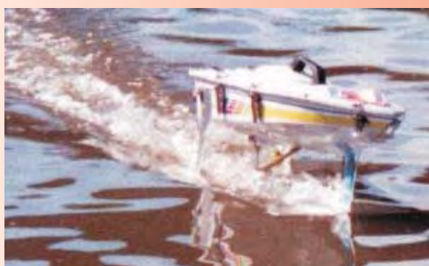
Malin Dixon's Design with Fully Submerged Hydrofoils and ACS
