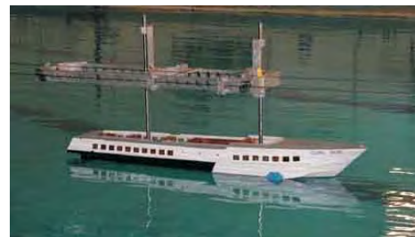
1:20 scale Rodriquez RHS 140 'Curl Curl' model suspended below towing rig, Australian Maritime College (AMC) Wave Wake Measurement Facility, Survival Centre.
