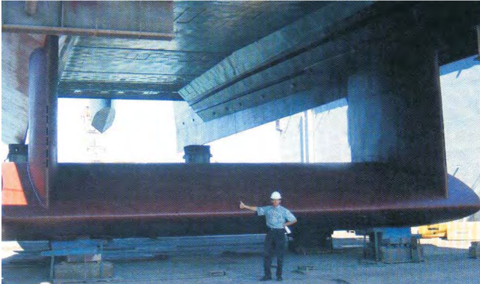
The Navatek-designed lifting body was installed beneath the hulls of the former SES-200
