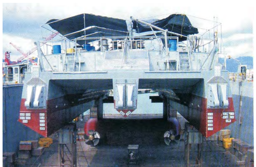
The lifting body houses the drive train: engines, gearboxes, shafts, and propellers
