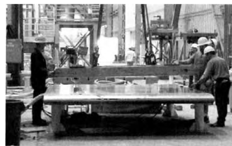
The front section of the HiPlate, showing the elliptical leading edge of the section. Photo by Bob Reiss,
