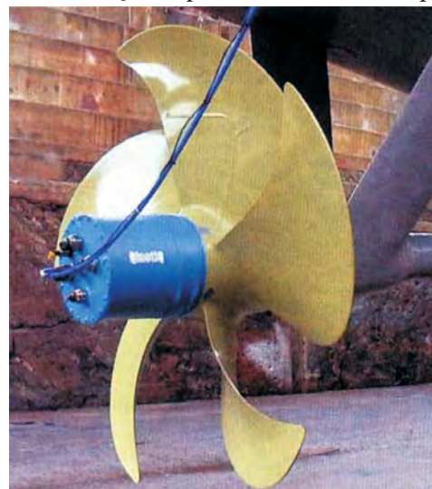
Qinetiqs composite propeller pictured on the trimaran Triton
