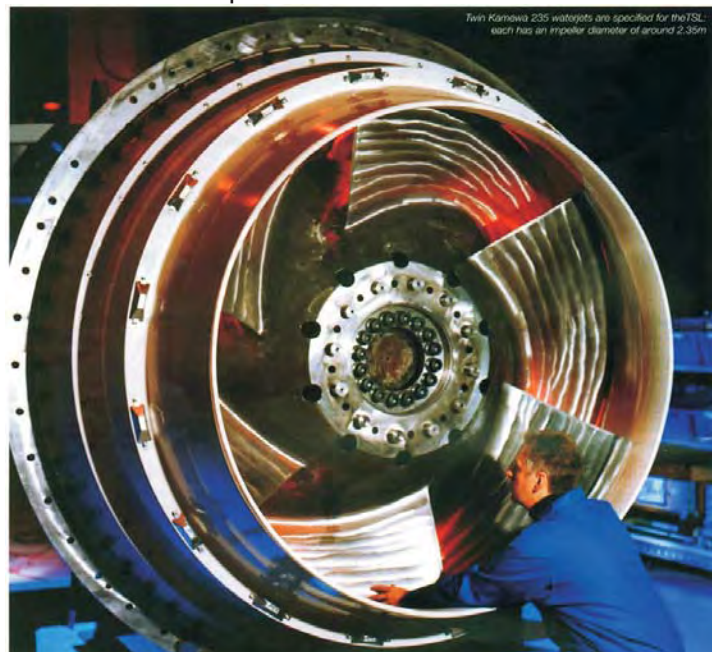
Twin Kamewa 235 WJ are specified for the TSL. Each has an impeller diameter of about 2.35 m.
