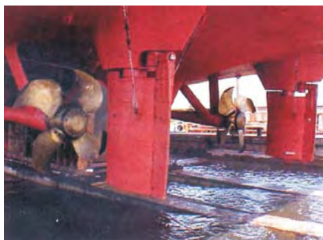
CLT blades installed on Superfast Levante
