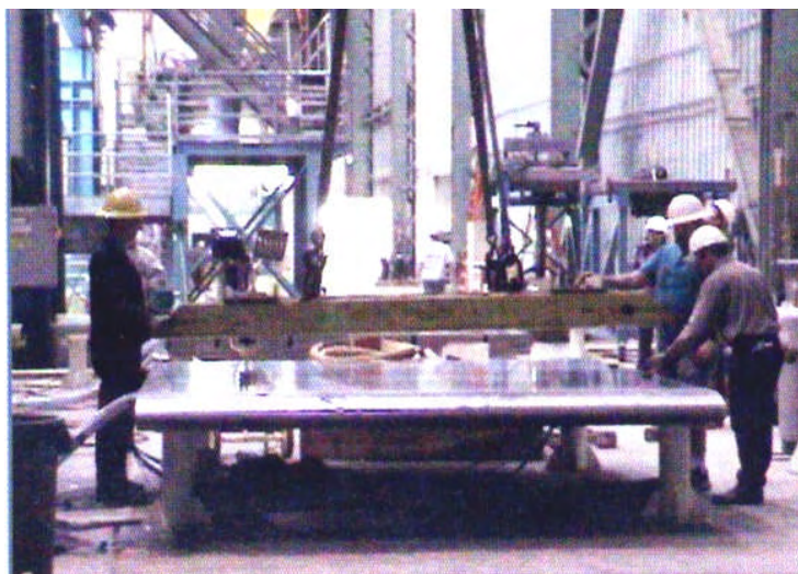
LCC Technicians Prepare Drag Reduction Experiment Plate for Insertion into Test Section of LCC
