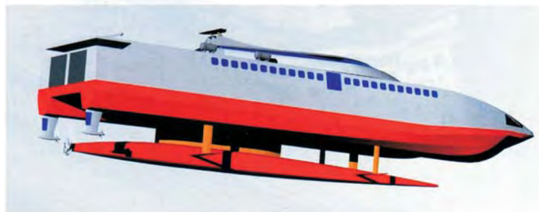
The AliSwath Concept Combines A Torpedo-Like Hull and Fully Submerged Foils
