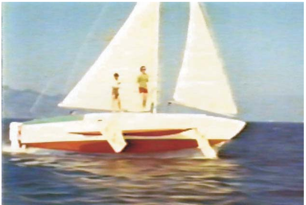
Side view of Williwaw showing sweep of the side and bow foils
