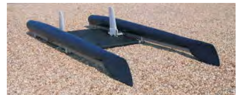
Inflatable Hulls (Turned Upside Down to Show Dagger Boards)
