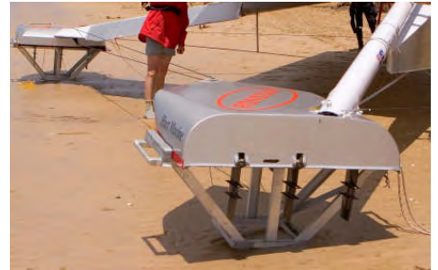
Macquarie Innovation Supported on Cradles While out of the Water. This Shows the Positioning of the Foils on each of the Pair of Planning Pontoon. Photo via Macquarie Speed Sailing Team.
