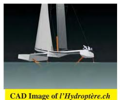
*l'Hydrotpère.ch* aims to validate the choice of this new geometry as well as permitting the effects of numerous parameter combinations to be evaluated based on the boat's performance. The boat will serve as a floating laboratory, equipped with systems that will enable a multitude of adjustments whilst sailing and multiple sensors enabling performance and load measurements to be made. The technologies tested on *l'Hydroptère.ch* should be transferable to the maxi.
