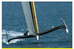
USA Frontal View Showing C-Shaped Daggerboard Retracted On Windward Side And Lowered On Lee Side
