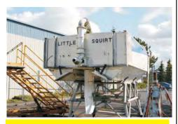
Stern view shows the jet that spews 3,600 gallons per minute. The water intake is a rectangular opening at the bottom-front of the strut (not in view).
