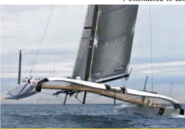
Alinghi 5 sailing with straight centreboards as seen retracted on the windward hull
