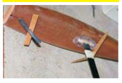
Figure 3: Towing model with Canting Keel. Note Foils on Centerline in this Case.
