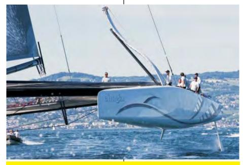
An S-shaped centreboard fitted to *Alinghi 5* shown in the retracted position on the windward hull
