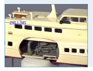
Left: This cutaway model shows the location of the starboard engine and its inclined mounting. (model photo ©Museum Victoria).
