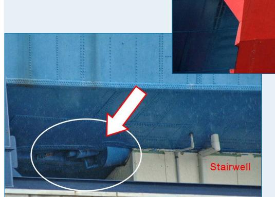
Left: Indicated is the starboard propeller shaft stern tube (the shafts have been removed). As seen in the following model photo, there are two shafts, each turning a propeller aft of the foil. Each shaft was powered by a 1350 hp German MB 820Db turbocharged after-cooled 12V cylinder diesel engine made by Mercedes-Benz.
