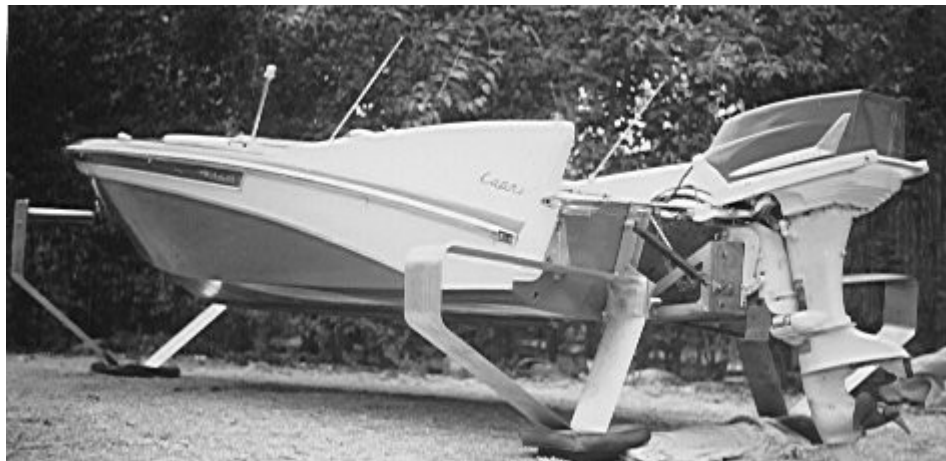
Figure 3. One of the first all-aluminum hydrofoil designs is shown mounted on an existing fiberglass boat. With a 40 hp Scott Atwater outboard motor, this boat achieved a speed of around 39 mph.
