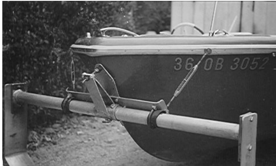
Figure 4. The handmade mount for the bow hydrofoil has the basic features of the later production kit. The bow foil is attached by four bolts. Note the angle adjustment plate and threaded rod positioned above the center of the cross tube.
