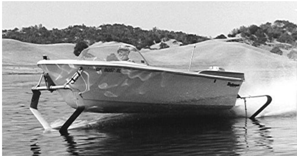
Figure 10. Hydrofoil boat equipped with the production Up-Right Hydrofoil kit. This boat achieved a speed of 47 mph with a 65 hp Mercury outboard, and could carry six people.
