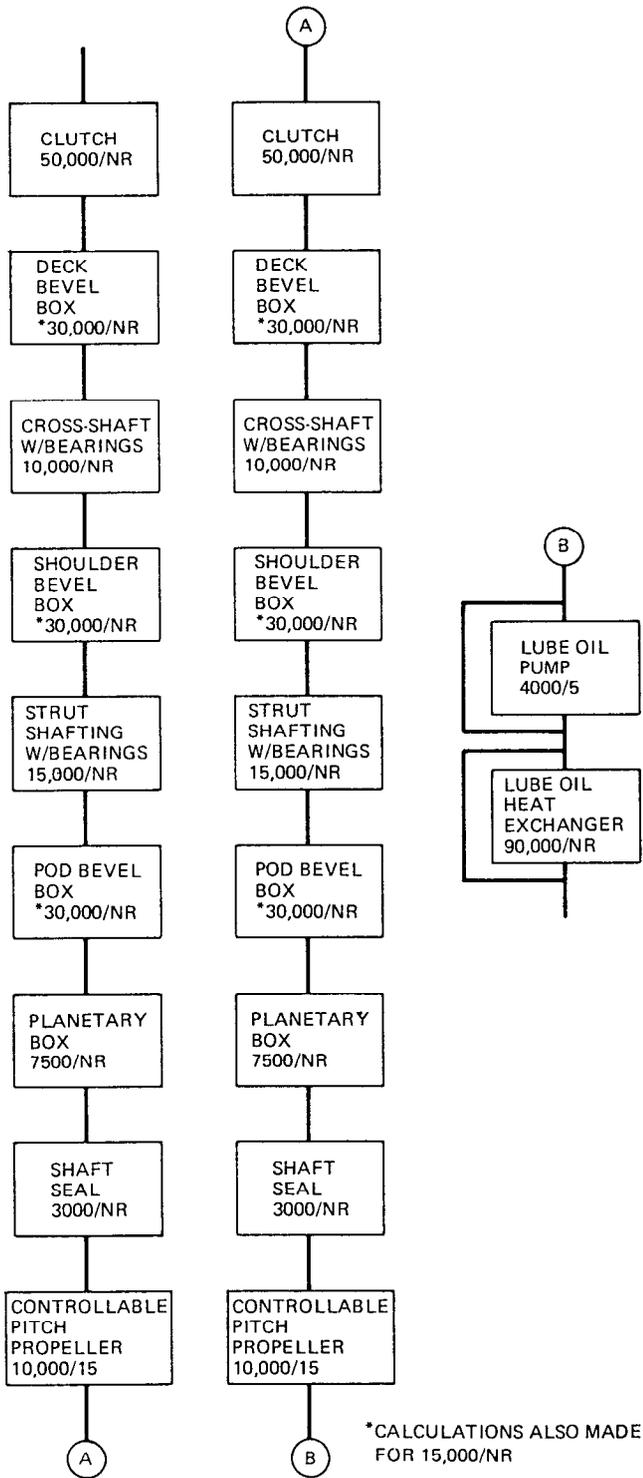
Fig. 7 Dual Mesh Mechanical Transmission Reliability Block Diagram - Foilborne Mode
