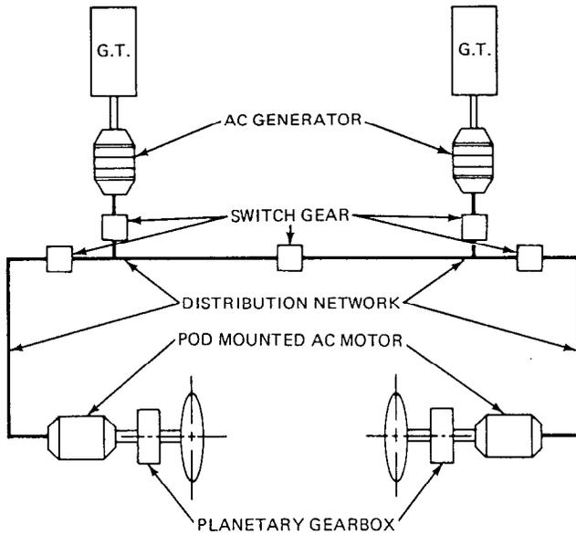
Fig. 4 AC Electric Transmission System
