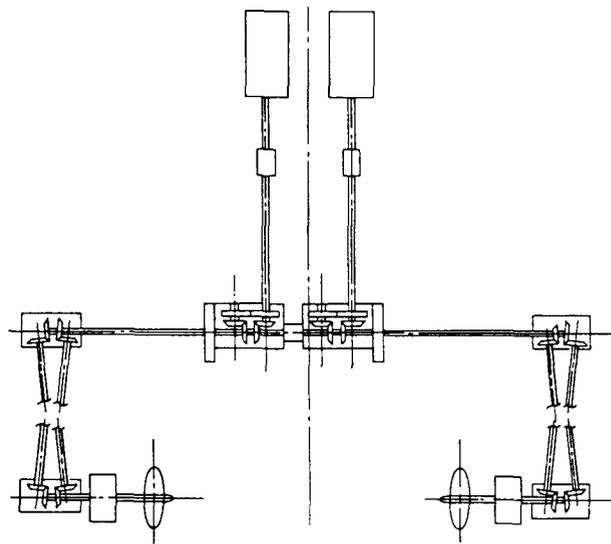
Fig. 2 Dual Mesh Transmission
