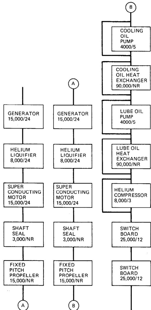
Fig. 10 DC Superconductive Drive Reliability Block Diagram - Foilborne Mode
