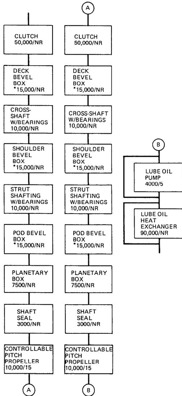
Fig. 8 Single Mesh Mechanical Transmission Reliability Block Diagram - Foilborne Mode
