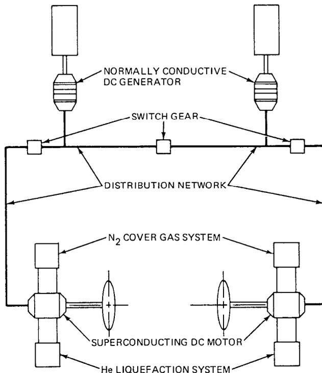
Fig. 5 Superconductive DC Transmission System
