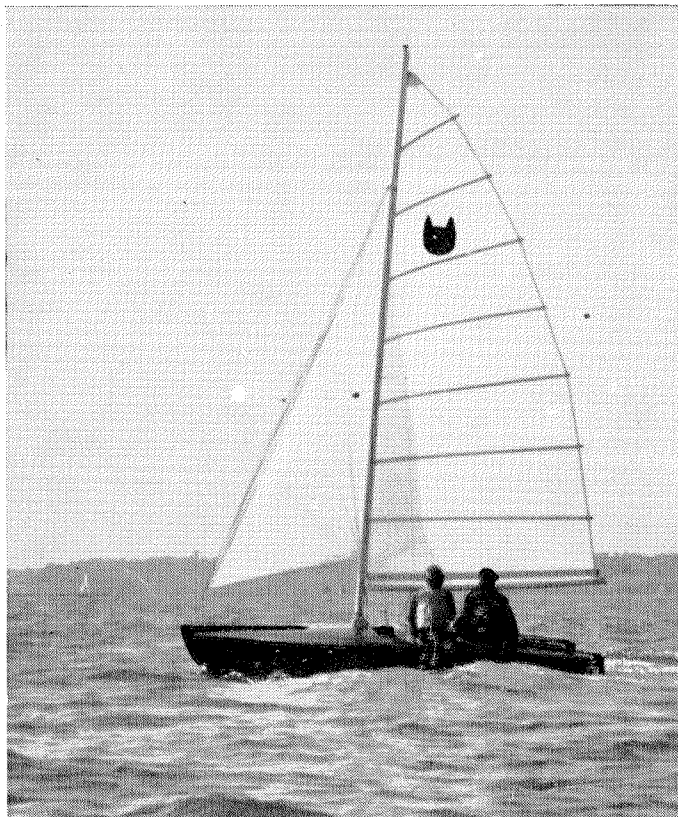
A 1959 Catamanner with fully battened sails, light alloy rotating mast and luff-spar. Designed by Erick J. Manners, M.I.E.I., A.M.B.I.M., A.M.I.W., Naval Architect
