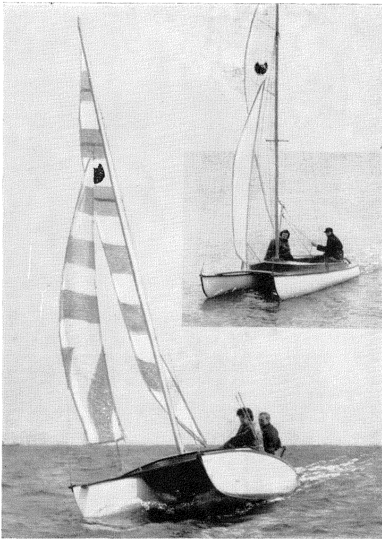
The small inset shows a photograph taken in 1957 of the 18 ft. 6 in. De Luxe Cruising model. The larger picture shows a similar size Catamanner fitted with optional hydrofoils to provide partial lift. These modified hydrofoils may also be fitted as and when required to the 14-ft. Racer Class Catamanner described in Chapter 9. Unless driven by outboard motor the 'Mannerfoils', as they have already been called, are only intended to give partial lift to sailing boats by creating a combined force to windward to reduce leeway plus an upward lift component to increase speed and steadiness. The first two Hydrofoil assisted sailing catamarans ever to be exhibited were shown at the 1959 National Boat Show. Editors were informed but they excited no comment.
