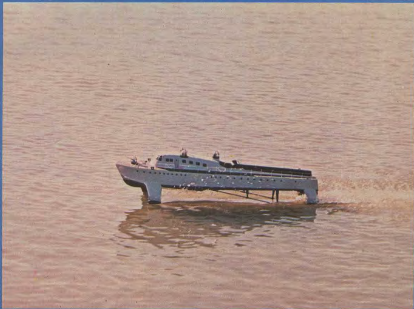
The VS 8 in the process of coming down off her foils. The boat simply mashes back down in the water. For all of the spray it kicks up, the VS 8 is a very dry boat in terms of the water it takes aboard.
