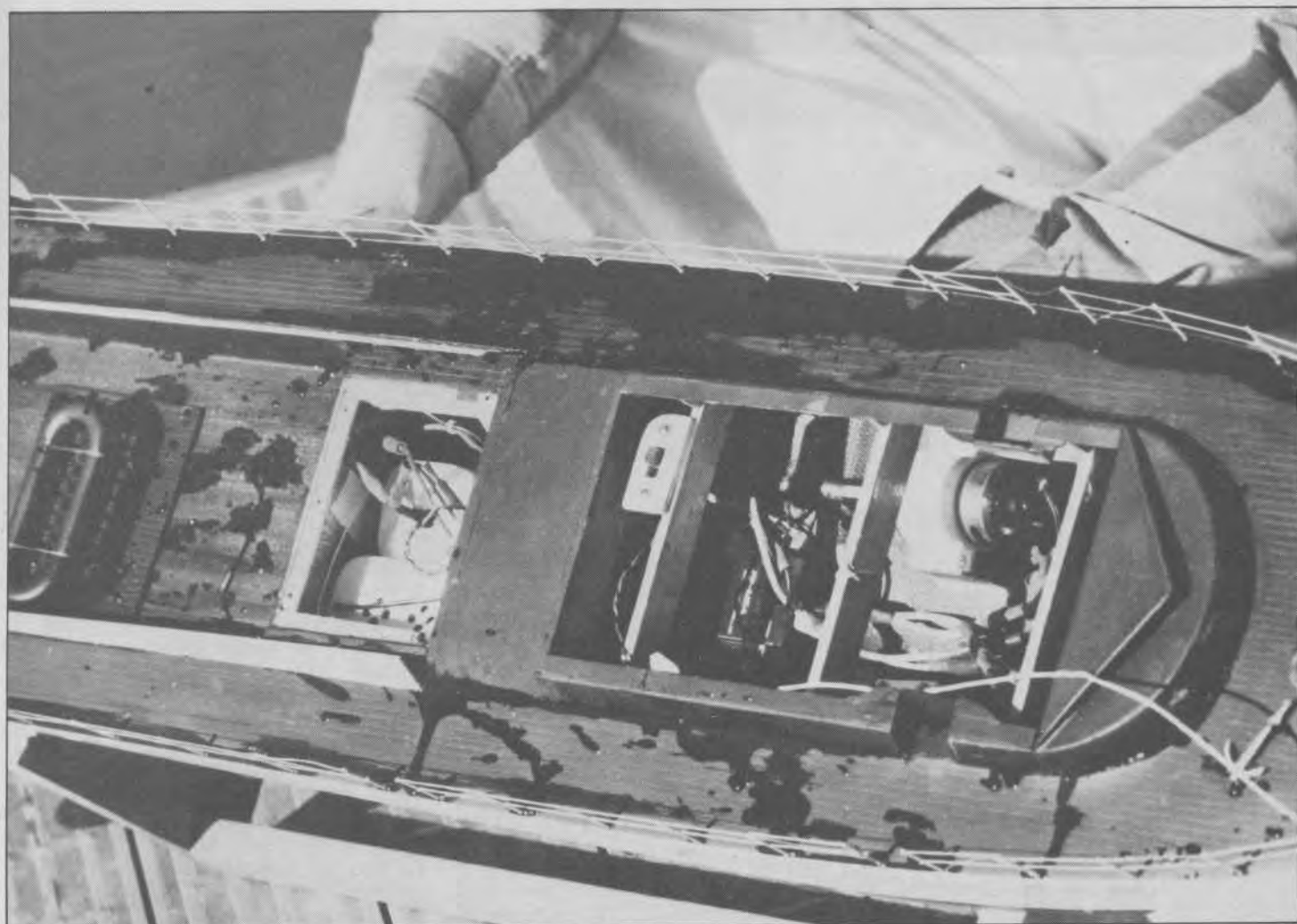
A look at the interior works of the prototype VS 8 model shows the two AstroFlite motors mounted well forward to accommodate the long drive shafts. Next comes the radio gear followed by the battery pack which is set in its own quick access compartment for fast changes. On the day we ran, two packs were used, one charging while the other ran. With this arrangement, you could literally run all day interrupted only by the two minute operation of switching packs in and out of the boat.
