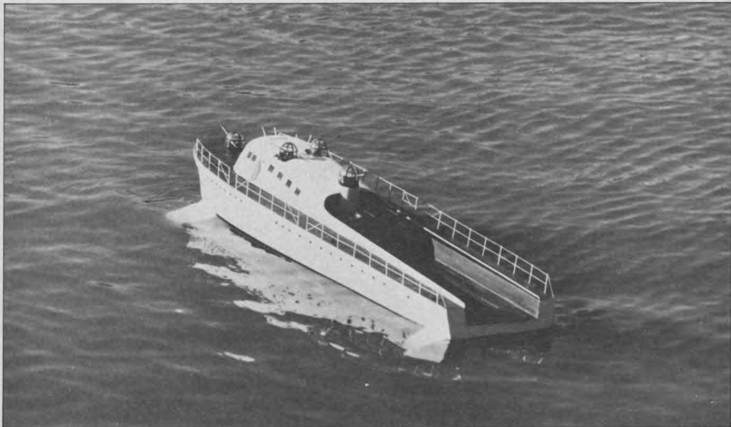
The VS 8 as seen from a profile view while running foilborne in the proper configuration (i.e., the majority of the foil surface under water is for maximum stability).
