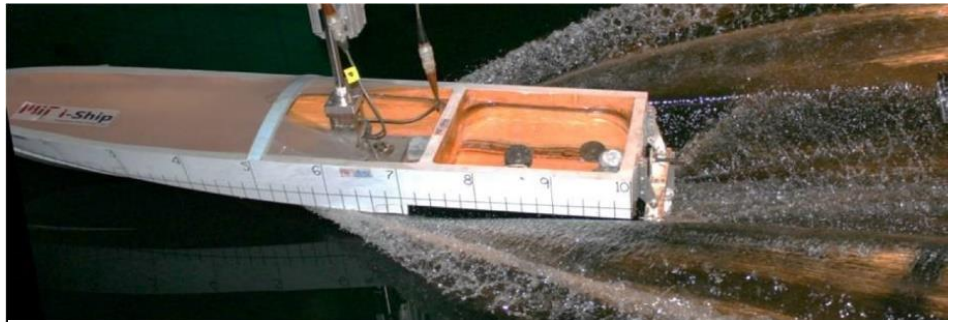
Model Test of Stepped Cambered Planing Hull with Hydrofoils (SCPH2)
