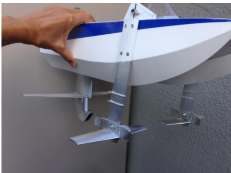
Close-Up of Foils on Model
