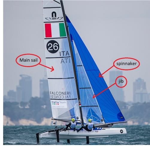
Figure 2: Nacra 17 sailing downwind with the main sail, the jib and the spinnaker in Auckland for the World Championship, 2019 ©Sailing Energy
